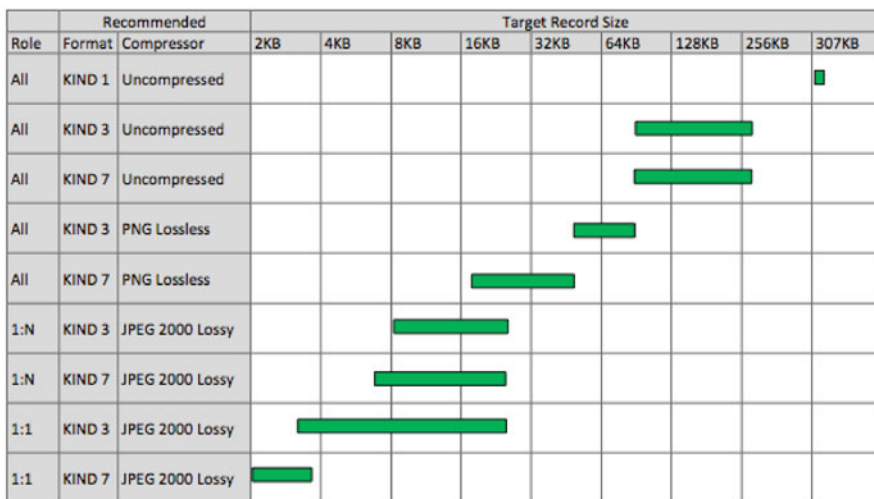
Fig. 3.7 Application-specific recommendations on compression and format from the IREX I evaluation
