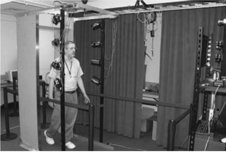
Fig. 13.29 Image acquisition setup for the Iris on the Move system (Image source: Matey et al. [17] ©IEEE)
