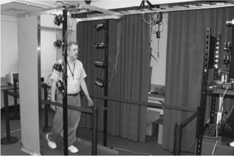
Fig. 14.1 Image acquisition setup used by the Iris On the Move (IOM) system (Image source: Matey et al. [8]. ©IEEE)
