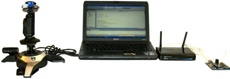
Fig. 7.5 The supervisory ground station. From left to right: joystick, PC, 801.1n wireless link, XBEE09P data link
