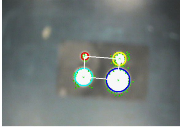
Fig. 6.2 Image processing for homography estimation: Detection of the four circles and parallel lines verification
