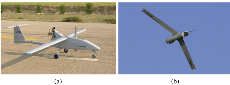
Fig. 1.10 Close-Range and Mini UAVs: (a) Aeronautics Ltd "Aerolight"; (b) Insitu and Boeing's "ScanEagle"
