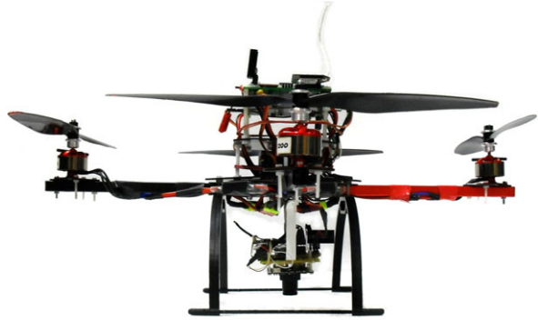
Fig. 6.3 The four-rotor aircraft experimental platform with the camera pointing downwards
