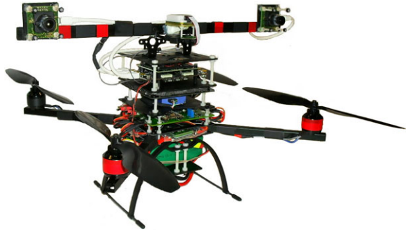
Fig. 7.1 The quad-rotor robotic platform equipped with a stereo imaging, inertial, and altitude sensing system
