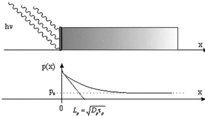
**Fig. 2.12** Representation of a semiconductor bar with an incident light on the lateral surface that causes charge injection: the charge concentration relaxes with spatial constant  $L_p$ , for  $x$  sufficiently far from the injection zone the equilibrium concentration is restored
