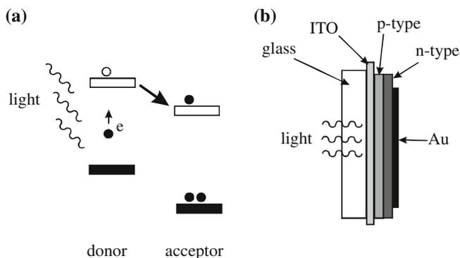
**Fig. 2.17** Electron transfer from donor to acceptor material (a), section of an organic cell (b)
