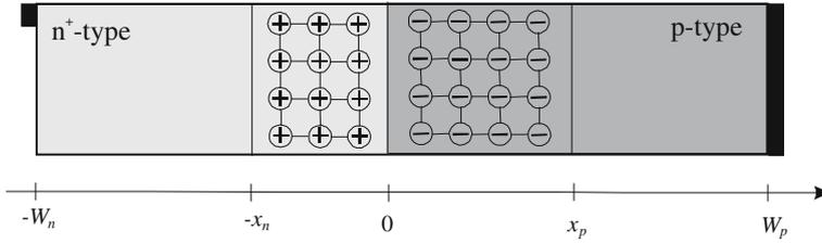
**Fig. 2.13** Schematic representation of a p–n junction
