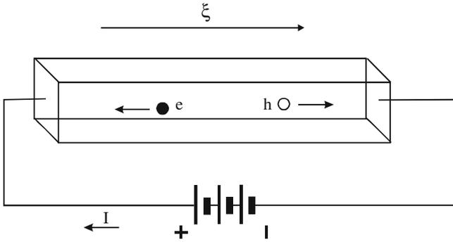
**Fig. 2.10** Semiconductor with electric field applied: a drift current formed by holes and electron occurs
