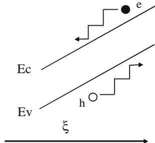
For a semiconductor whose length (corresponding to the  $x$  direction) is bigger than the other two dimensions and the electric field is in the  $x$  direction. A one-dimensional (1D) representation can be used, as depicted in Fig. 2.10; Eq. (2.30) becomes:
