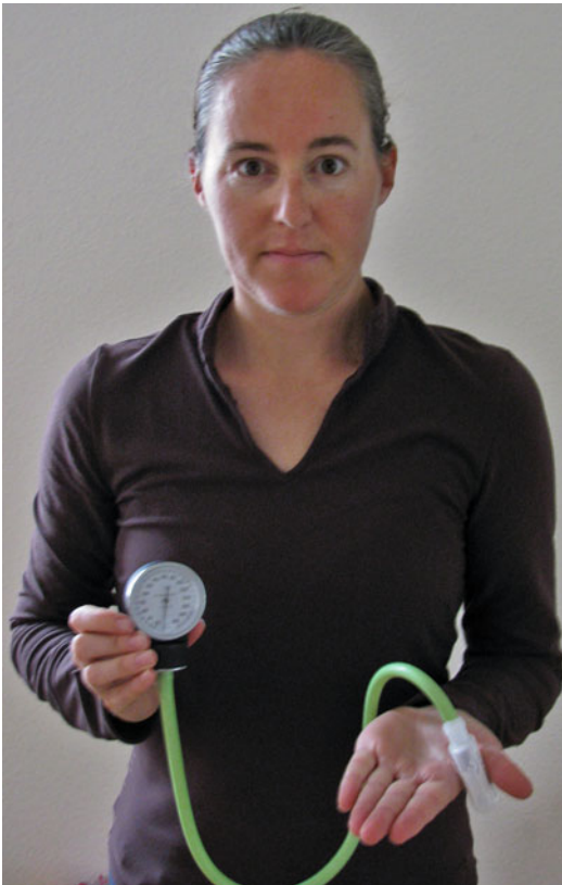
Fig. 23.3 The Thumbometer™ is constructed using a half ounce eye drop like bottle connected by a piece of Theratubing to the sphygmomanometer from a standard manual blood pressure cuff (Courtesy of Peter Edgelow)
