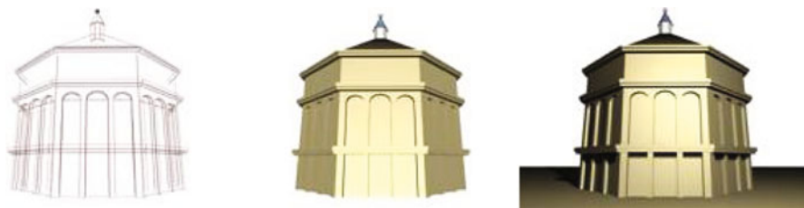
Fig. 7.6 Left: Hidden-line rendering. Middle: Flat-shaded rendering. Right: Shadow-mapped rendering
