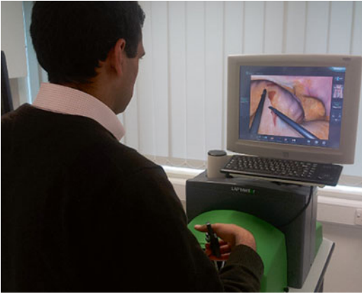
Fig. 43.3 Example of a virtual reality simulator. The trainee is using a robotic interface that translates the movements of the surgeon into motion within a virtual reality environment. Haptic feedback to the instruments can enhance the perceived level of reality
