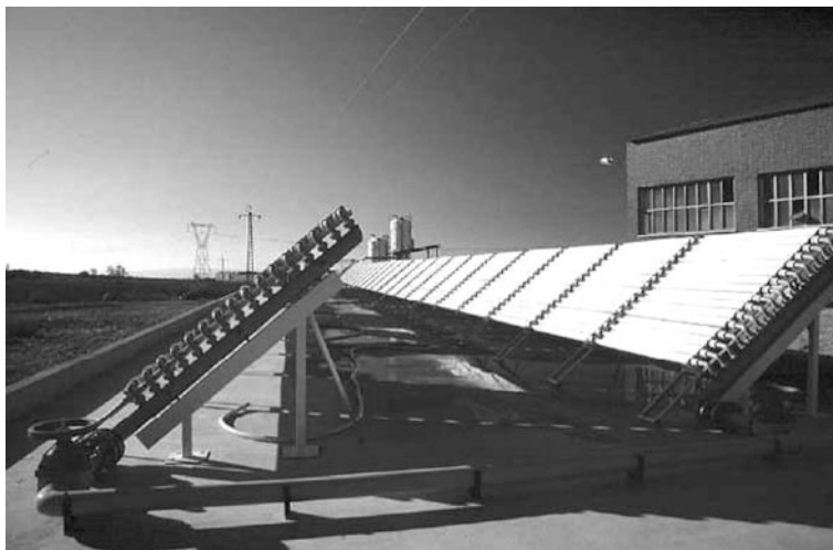
Fig. 6.5 Compound Parabolic Collecting Reactor (CPCR) at the Plataforma Solar de Almería (PSA) [218]
