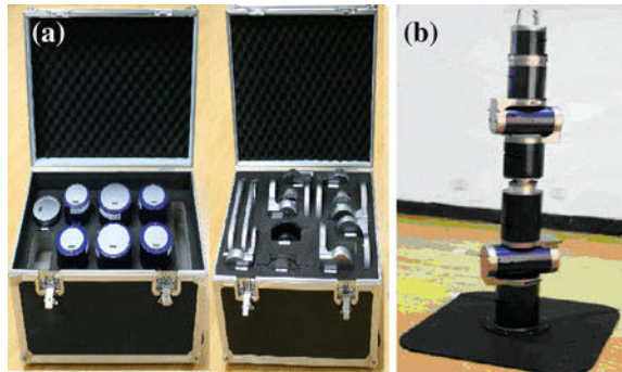
Fig. 49.1 Module library and a 6-DOF configuration. a Module library. b A 6-DOF configuration
