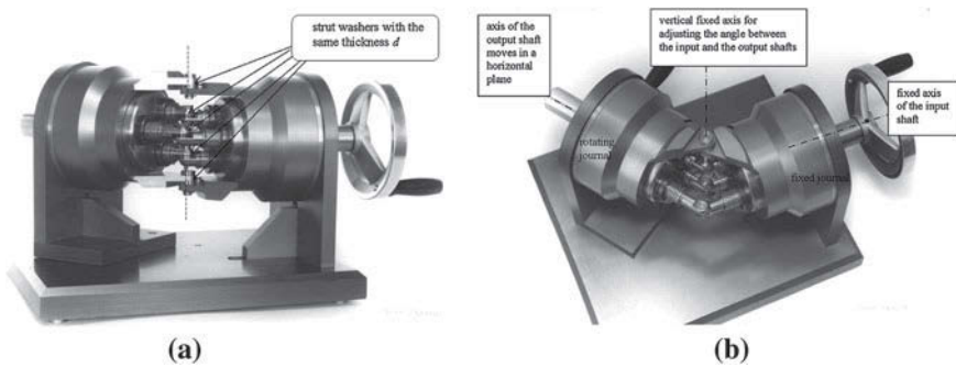
Fig. A.1 A new patented homokinetic joint
