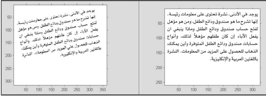
Fig. 7.6 Illustration of a skew corrected image of text. (Left) Before skew correction. (Right) After skew correction
