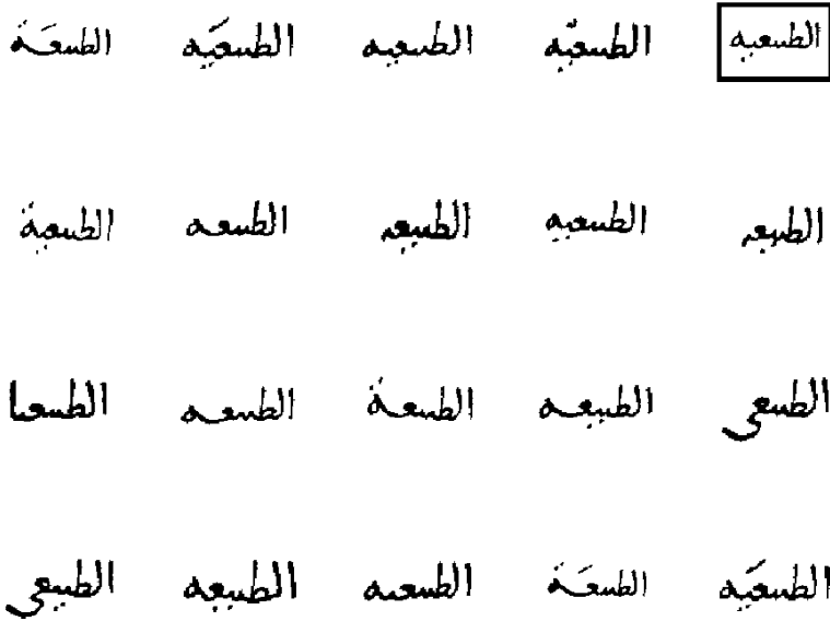
Fig. 19.14 A graphical query is shown (in a box ), along with a few of its spotted instances. The ability of the system to tolerate writing variations and the presence of dots can be seen from the spotting results
