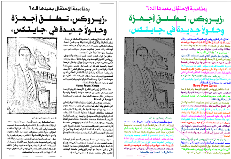
Fig. 2.3 A sample newspaper image printed in Arabic Naskh script and its corresponding layout analysis result: gray region represents non-text components, color-coded labeling represent segmented text lines, and magenta line shows text line reading order. [Note: left image has been taken from the website [17]]
