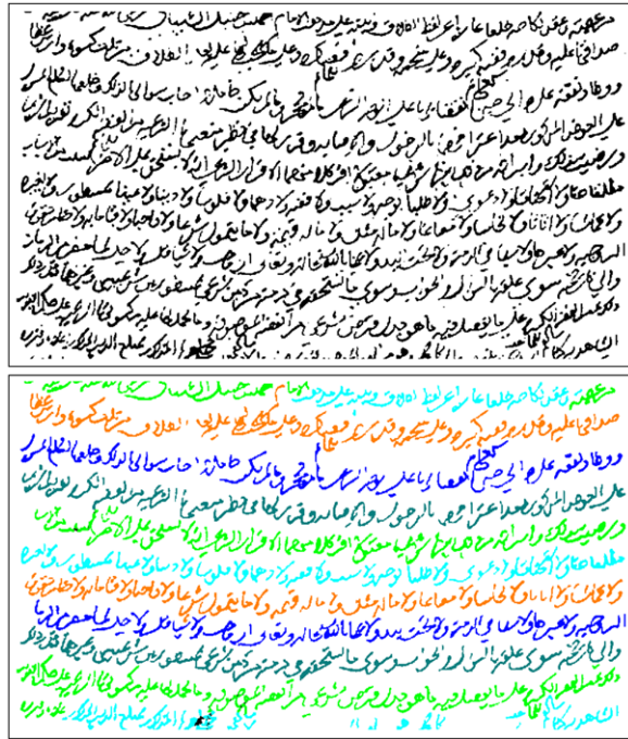
Fig. 4.8 Above: Binarized image after background normalization. Below: Text line separation using the binarized image
