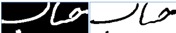
Fig. 11.7 Black background image at left shows the dilated image of the white background image at right . They both show the word Account in Farsi
