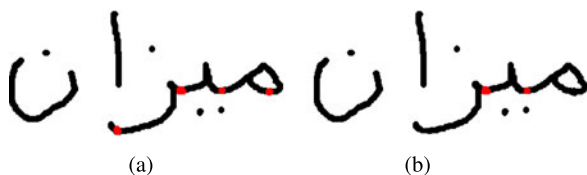
Fig. 1.13 Segmentation of the first component of the word “meezan.” (a) All local minima, (b) valid segmentation points
