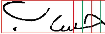
Fig. 11.8 The word “Account” is shown in the figure. Red and green windows are consecutive and the 50 % overlap is shown
