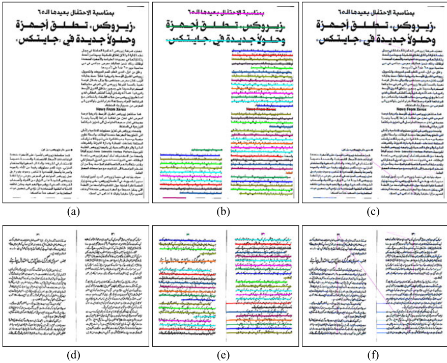
Fig. 2.11 Example images illustrating results of reading order for a newspaper and a book page. Thin horizontal lines with different colors indicate detected text line segments, and the magenta lines running down and diagonally across the image indicate reading order
