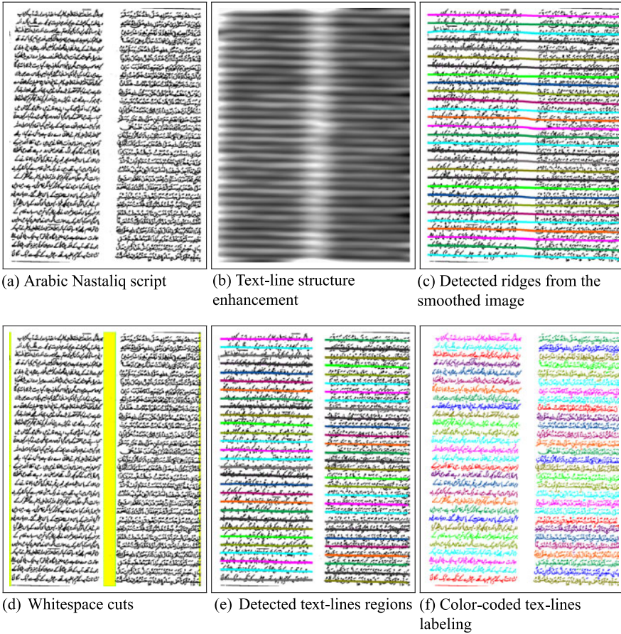
Fig. 2.9 Steps of the ridge-based text line finding algorithm. (a) An example image of Arabic Nastaliq script. (b) Smoothed text line (text lines enhanced) image, which is generated by using oriented anisotropic Gaussian smoothing filter bank approach. (c) Detected ridges from smoothed image using Riley-based ridge detection [33, 34] algorithm. There are over-segmentation errors because of multi-column format. (d) Column separators that were detected through whitespace analysis; these separators help in correcting over-segmentation errors. (e) Processed ridges using whitespace separators; each ridge covers a complete region of a particular text line. (f) Color-coded labeled text lines result using detected ridges
