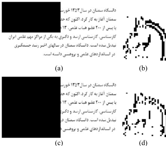
Fig. 13.15 Effect of occlusion on the fractal watermarking. (a) Document with 25 % occlusion. (b) Decoded watermark. (c) Document with 50 % occlusion. (d) Decoded watermark
