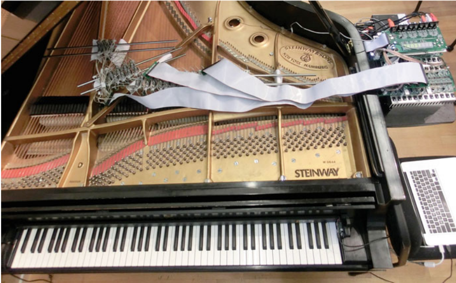
Fig. 7.10 The magnetic resonator piano, an electronically-augmented acoustic piano. Electromagnets induce the strings to vibration in response to continuous gestural input sensed from the motion of the piano keys
