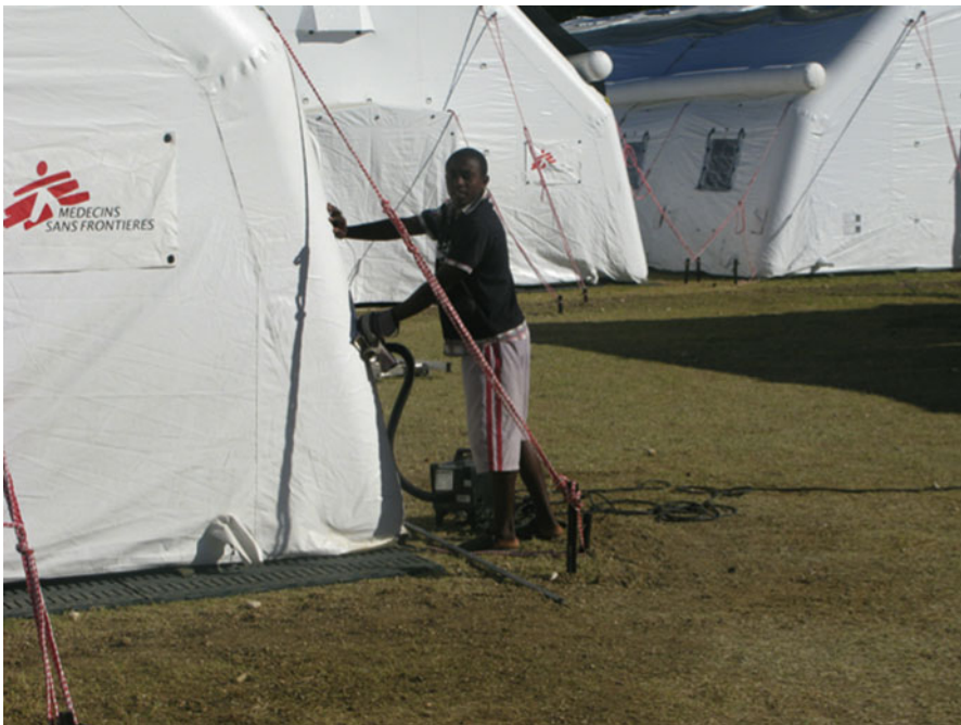
Fig. 33.7 Compressed air to top up the tents
