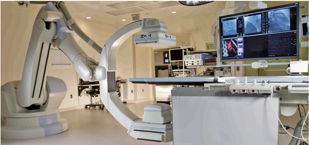
Fig. 1.3 Artis zeego multi-axis imaging system. Artis zeego multi-axis imaging system (Siemens, Erlange, Germany)
