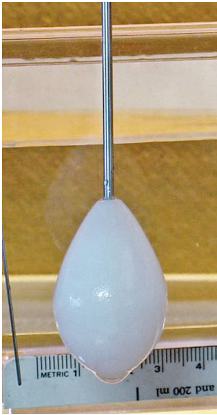
Fig. 65.3 Ice ball formation on a cryoneedle
