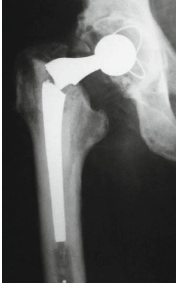
Fig. 23.5 Cemented stem breakage 2 years after implantation. Excellent cement mantle
