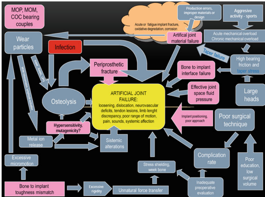
Fig. 23.2 A simplified overview of modes of failure affecting artificial joints
