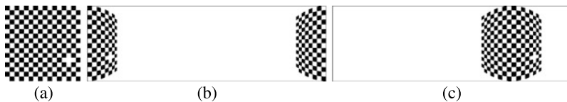
Fig. 9.2 (a) A planar image of dimensions 256 \times 256 and its corresponding cylindrical images (b) when \theta_0 = 0 and (c) when \theta_0 = \pi/2 in clockwise direction (or -\pi/2 in counter-clockwise direction). In these examples, r = 128 , h = 256 , and f = 128 , all in pixels
