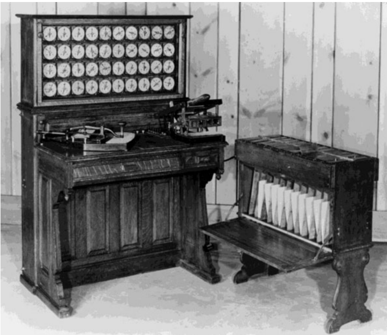
Fig. 6.2 Hollerith's tabulator (1890) (Courtesy of IBM Archives)
