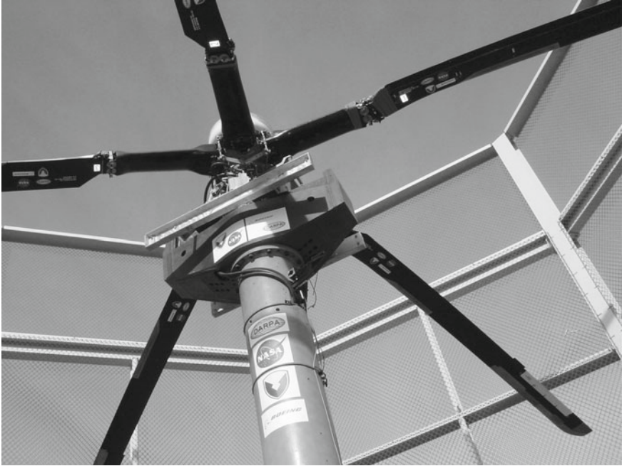
Fig. 1.4 A smart rotor blade undergoes whirl tower tests at The Boeing Company facility in Mesa, Arizona, USA [12]. For the purposes of control system design, the dynamic behavior of flexible and lightly damped structures such as active rotor blades can be effectively emulated by much simpler laboratory models
