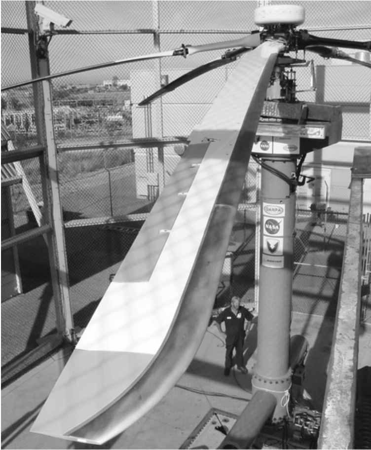
Fig. 5.2 From the control engineering point of view a clamped cantilever beam has similar dynamic properties to helicopter rotor blades. The photograph shows an experimental smart rotor structure in a whirl tower test [10]
