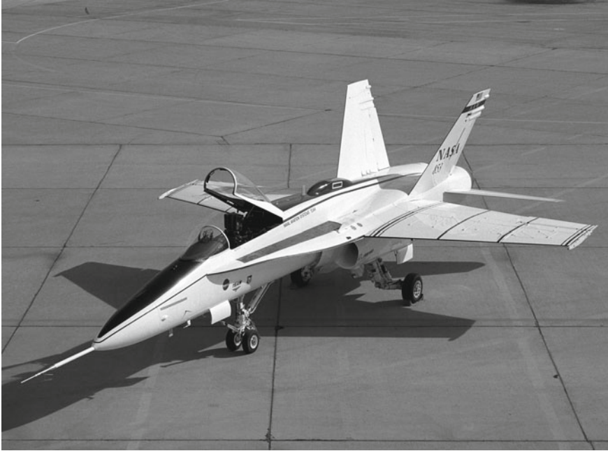
Fig. 4.1 An excellent example of the possibilities offered by active vibration control: a modified F/A-18A test aircraft with active aeroelastic wings [76] is shown with accelerometers visible on the wing surfaces. In addition, the actuators and sensors the performance of active systems depends on the choice and design of control algorithms as well (Courtesy of NASA)
