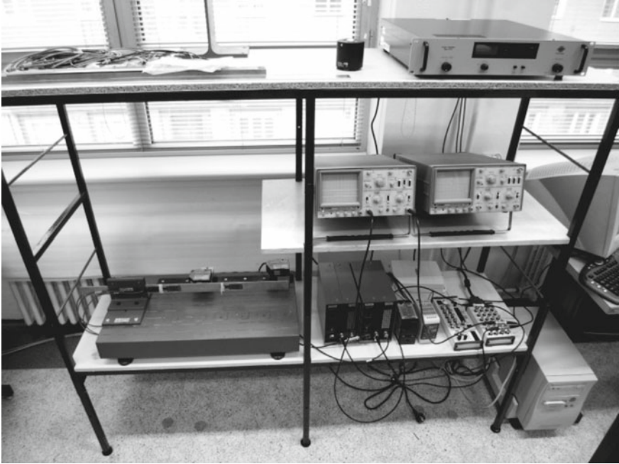
Fig. 5.4 Complete experimental setup for testing efficient MPC in vibration attenuation applications (excluding the Target PC used for real-time control and Host PC used for controller development)
