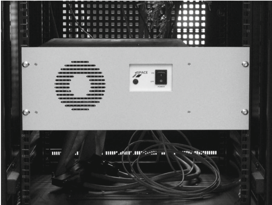
Fig. 8.1 Powerful rapid control prototyping systems with high memory capacity and computation speed are widespread in the automotive and aerospace industries. The proliferation of MPC controllers in practical applications is currently limited because of high computational costs. The use of model predictive control may be advanced not only by more powerful hardware, but better designed algorithms and strategies as well
