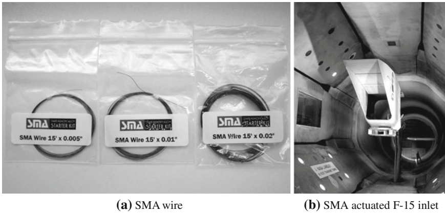
Fig. 3.8 Spools of shape memory alloy wires with different diameters are shown in (a), while (b) shows a full-scale F-15 inlet (modified flight hardware) with integrated shape memory alloy actuators installed in the NASA Langley Research Center 16-foot Transonic Tunnel [81]
