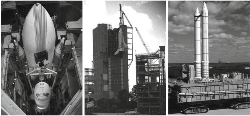
(a) Orbiter Enterprise in test stand installation (b) Removal of orbiter Enterprise from test stand (c) Mobile launcher platform and solid rocket boosters
