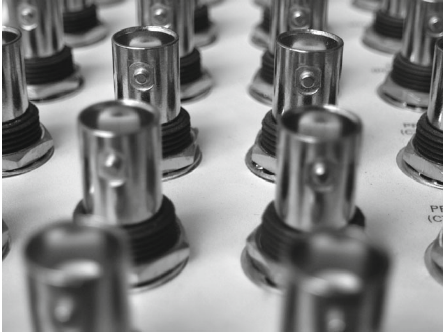
Fig. 5.1 The image illustrates an array of BNC connectors on a terminal, used for supplying analog inputs and outputs to the experimental demonstration hardware
