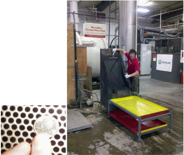
Fig. 14 Primary fungal harvesting also showing detail of screen openings
