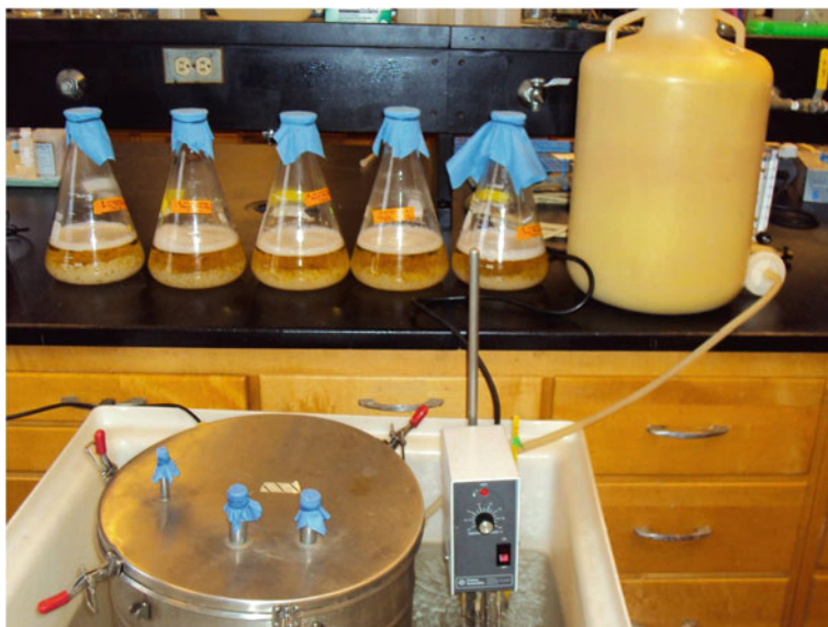
Fig. 13 Pre-culturing set-up for preparing pilot plant inoculum
