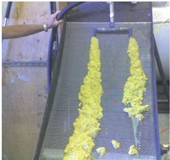
Fig. 15 Secondary screen dewatering equipment
