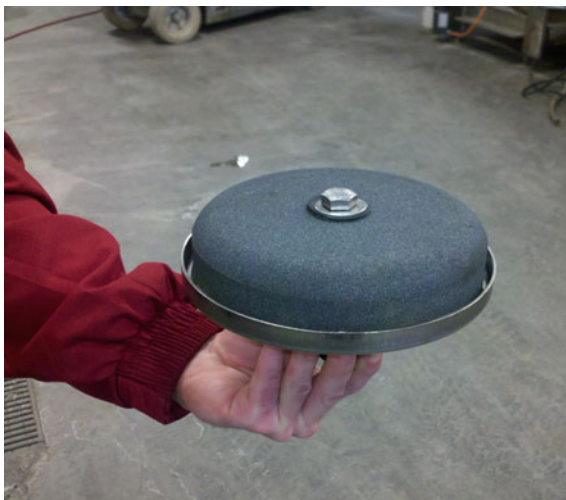
Fig. 12 Photo of one of the porous diffusers
