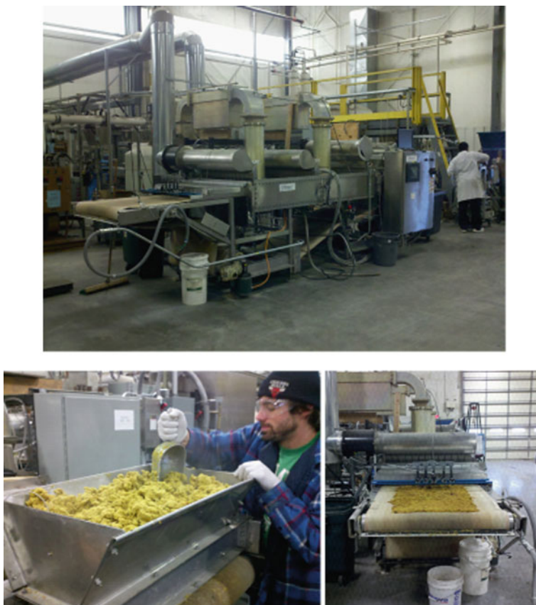
Fig. 16 Cellencor microwave dryer showing details of feeding the fungal biomass and the dried product emerging from the drying tunnel
