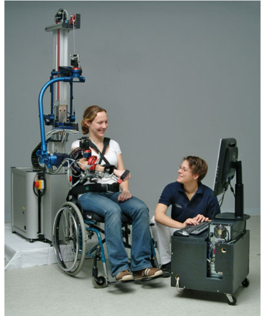
Fig. 9.1 Typical setup for a robot-supported arm therapy system
