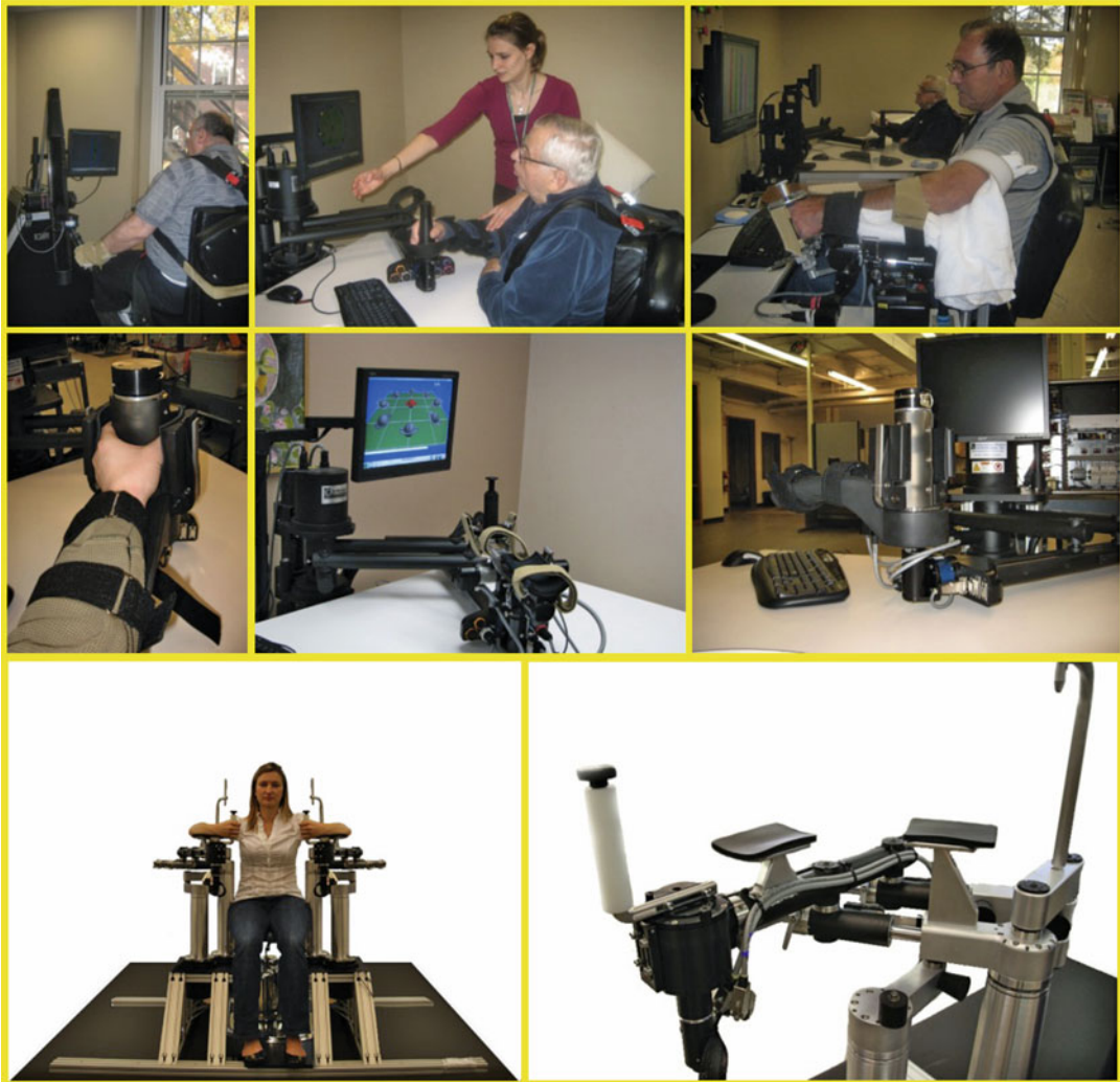
Fig. 8.1 A gym of upper extremity robots. Top row: left panel shows a person with chronic stroke working with the antigravity shoulder-and-elbow robot, middle panel shows a person working with the planar shoulder-and-elbow robot, and right panel shows the wrist robot during therapy at the Burke Rehabilitation Hospital. Middle row: left panel shows the hand module for grasp and release, middle panel shows reconfigurable robots. The robotic therapy shoulder-and-elbow and wrist modules can operate in stand-alone mode or be integrated into a coordinated functional unit; right panel shows the shoulder-
