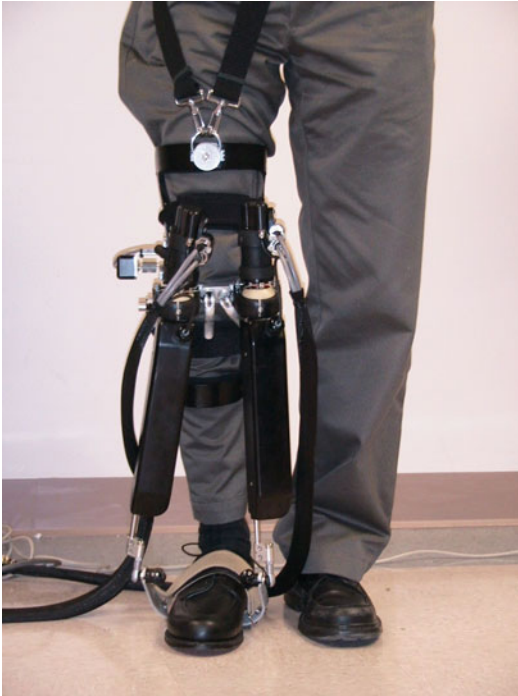
Fig. 22.1 AnkleBOT robot provides subjects active assistance in flexion–extension and inversion–eversion as they walk overground or on a treadmill
