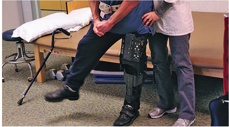
Fig. 22.3 Tibion robotic system applied to the knee of a patient with left leg hemiplegia
