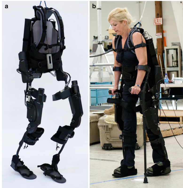
Fig. 22.4 eLEGS by Berkeley Bionics (Berkeley, CA, USA). (a) eLEGS is an exoskeleton actuated at the hip and knee joints while the foot is passively supported. (b) A patient walking in eLEGS (a – Courtesy of Berkeley Bionics; used with permission)
