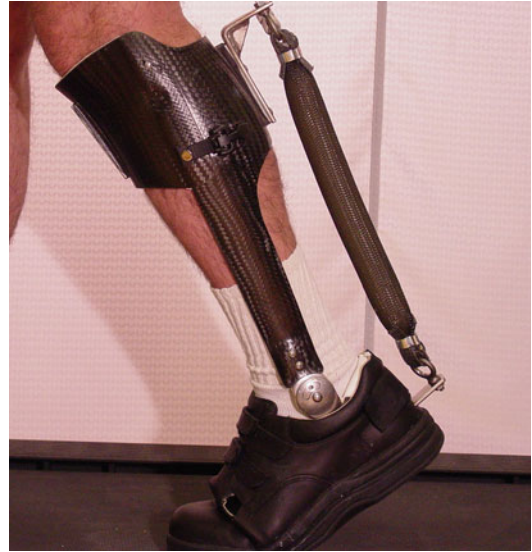
Fig. 22.2 Pneumatically actuated ankle device being tested to assist with limb propulsion [9]
