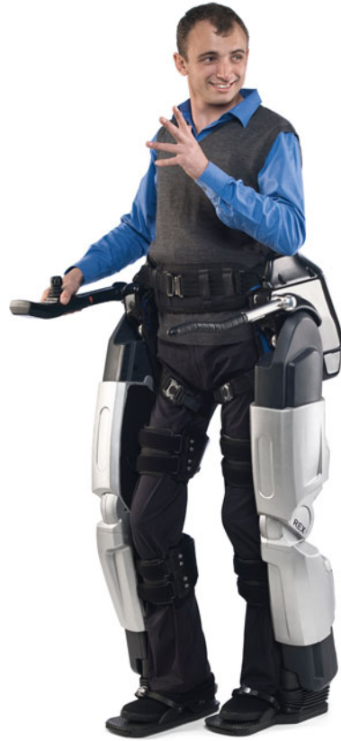
Fig. 22.5 Rex exoskeleton by REX Bionics (New Zealand) (Courtesy of Rex Bionics; used with permission)
