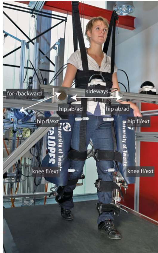
Fig. 21.1 Subject attached in the first prototype of the LOPES device. The eight actuated DOFs are schematically indicated
