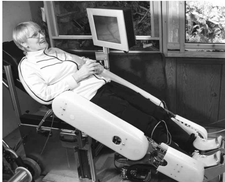
Fig. 2.3 The MoreGait is a pneumatically actuated robot for the training of ambulatory function. The device allows the use at the patient's home
