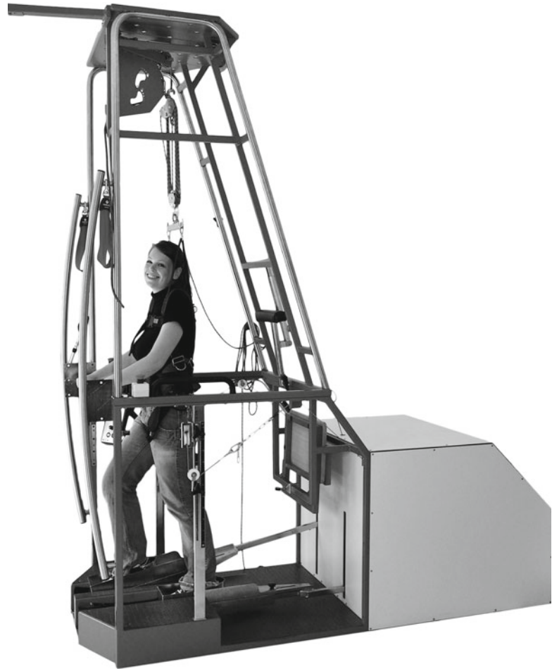
Fig. 2.1 The gait trainer GT I assists the patient during gait training using an end-effector-based approach combined with a system for partial unloading of the body weight (Photo courtesy Reha-Stim, Berlin, Germany. Used with permission)
