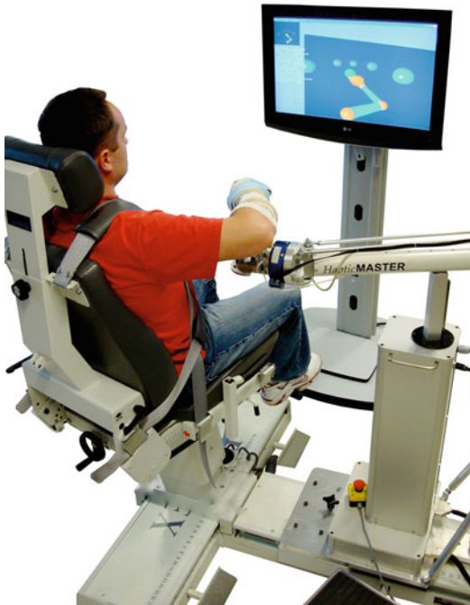
Fig. 19.4 Example of a research participant positioned with the ACT-3D showing the five reaching targets (From Ellis et al. [46]; used with permission)
