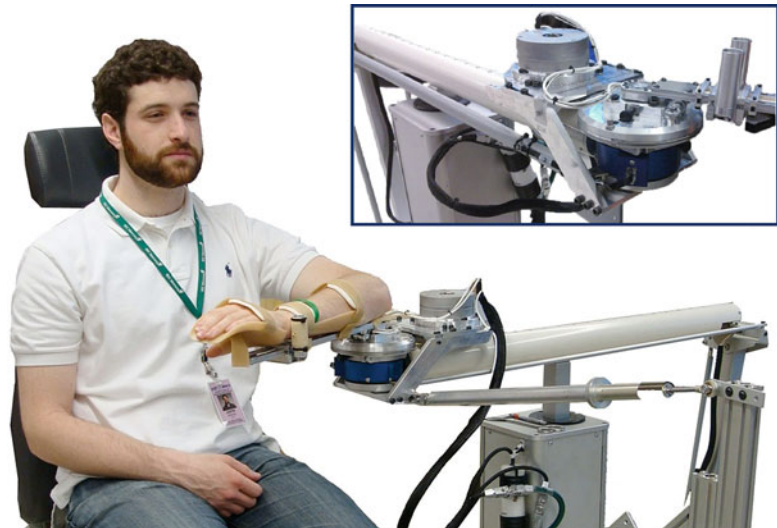
Fig. 19.5 The ACT-4D robotic device allows for single-joint perturbations at the elbow combined with adjustable shoulder abduction loading to study the relationship between synergies and abnormal stretch reflex or spasticity following brain injury
