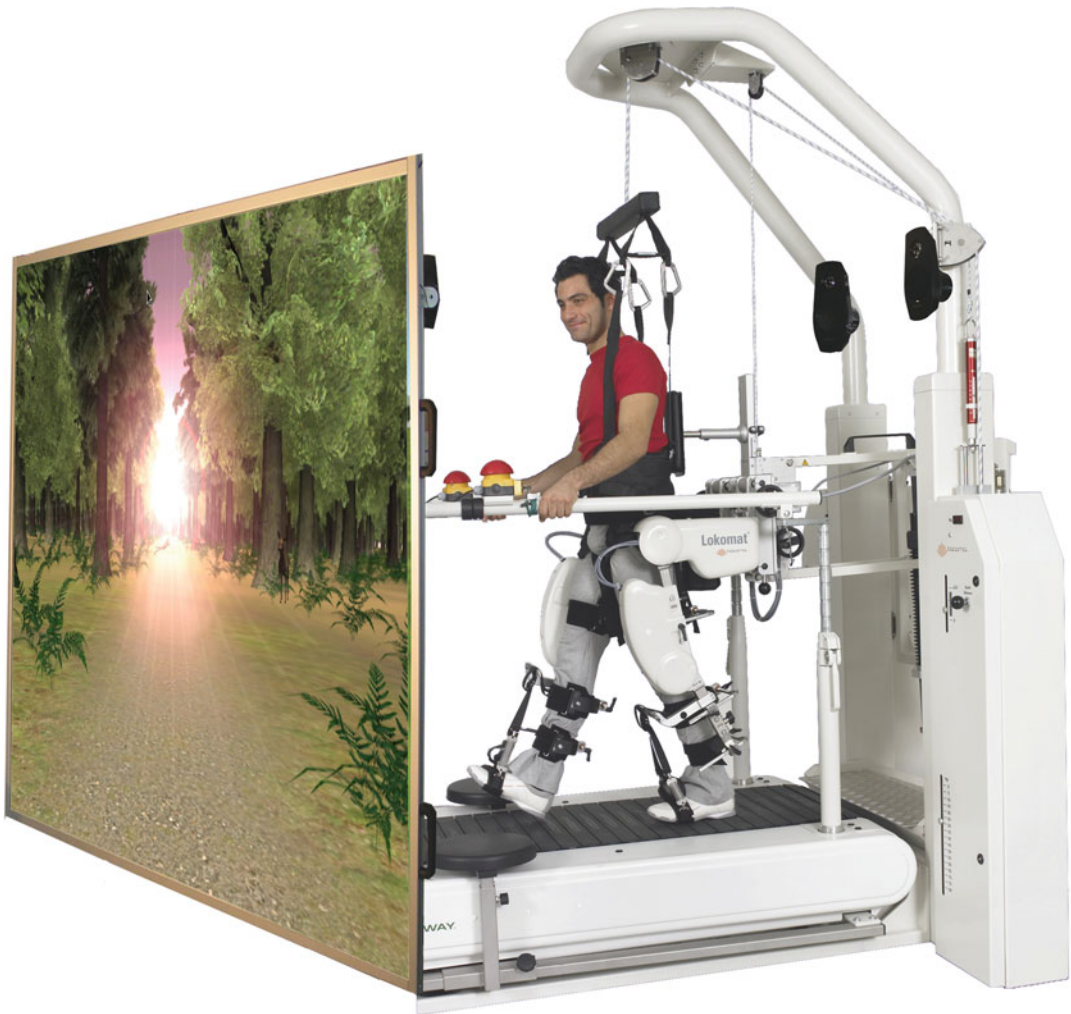
Fig. 13.5 Walking through a virtual environment. Lokomat in combination with a virtual reality back-projection display system (From: Riener et al. [31]. Used with permission)
