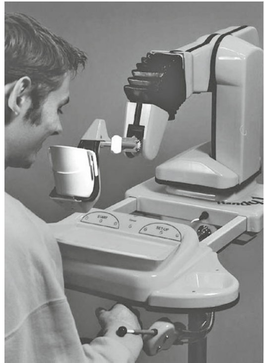
Fig. 11.2 The Handy 1 workstation, intended to help users with eating, drinking, and grooming. First developed by Mike Topping at Staffordshire University (Reprinted with permission from: Topping [92]. © Emerald Group Publishing Limited; all rights reserved)
