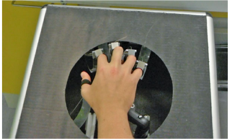
Fig. 11.4 HandCARE3 system. Cables attached to the fingertips can pull the digits open. The springs shown provide a restoring force to push the digits back into flexion when the pulling force is removed (Photo courtesy of Dr. Etienne Burdet of the Imperial College London)
