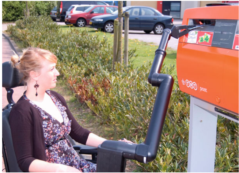
Fig. 11.3 The iARM wheelchair-mounted assistive robot, seen here assisting a user to mail a letter (Photo courtesy of Exact Dynamics, Didam, the Netherlands)
