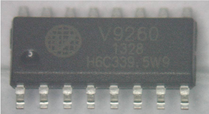
Fig. 34 Metering chip assembled in SOP16 package
