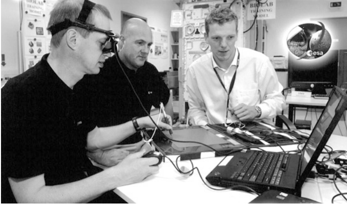
Figure 3.10. ESA Astronauts During a Training Session for the 3D-SPACE Experiment. This ISS Experiment Uses a Head-Mounted Visual Display, a Trackball, and a Digitizing Tablet. The Subject Is Presented with Depth-Related Visual Illusions, or 3D Objects That He Can Adjust So That They Look “Normal”, or Natural Scenes in Which He Has to Judge the Distance Between Identified Landmarks. The Digitizing Tablet Is Used for Neuropsychological Testing of Writing Horizontally and Vertically and Drawing Geometrical Figures with the Eyes Closed. (Credit ESA).
