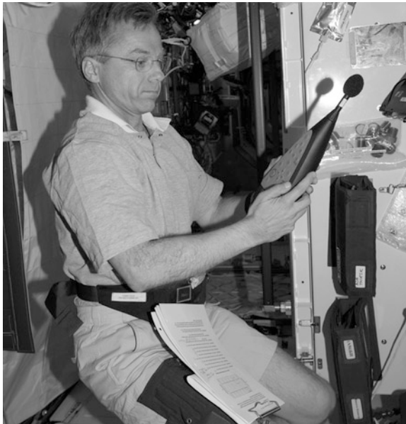
Figure 3.11. Canadian Space Agency Astronaut Robert Thirsk Works with a Sound Level Meter for an Acoustic Survey in the Destiny Laboratory of the ISS. Note the Procedure Documents on His Lap. (Credit NASA).
