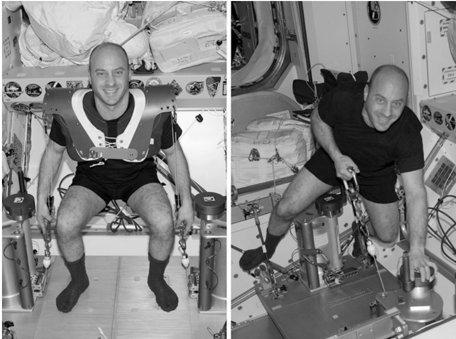
Figure 5.19. The Interim Resistive Exercise Device (iRED) on Board the ISS. The Astronauts Can Pull on a Cord to Create Resistance ( Right ), or Use a Shoulder Harness System to Do Deep Knee Bends, Which Stimulate the Anti-Gravity Muscles ( Left ). (Credit NASA).
