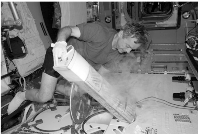
Figure 8.6. Astronaut Robert Thirsk Inserts Urine Samples into the Minus Eighty Degree Laboratory Freezer for ISS (MELFI) as Part of a Nutritional Status Assessment Study in the Kibo Laboratory of the ISS. (Credit NASA).
