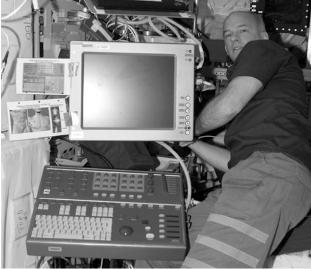
Figure 4.1. Astronauts Onboard the ISS Are Using an Ultrasound Machine to Perform Exam of the Heart and Other Internal Organs. Ultrasound Probes Send High-Frequency (Megahertz) Sound Waves into the Body. Because Sound Waves Travel Through Each Organ, or Tissue, at a Different Speed, the Probe Is Able To “See” What the Reflected Sound Waves Have Found. (Credit NASA).
