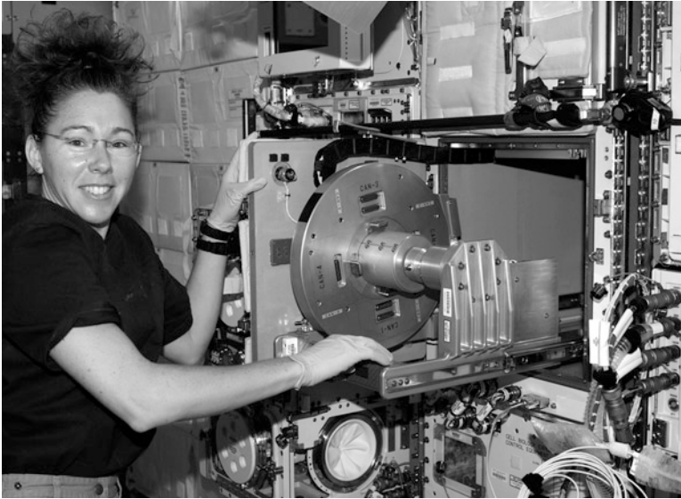
Figure 2.28. A Crewmember Conducts a Biology Experiment Facility in the Saibo rack in the Kibo Laboratory of the ISS. (Credit NASA).
