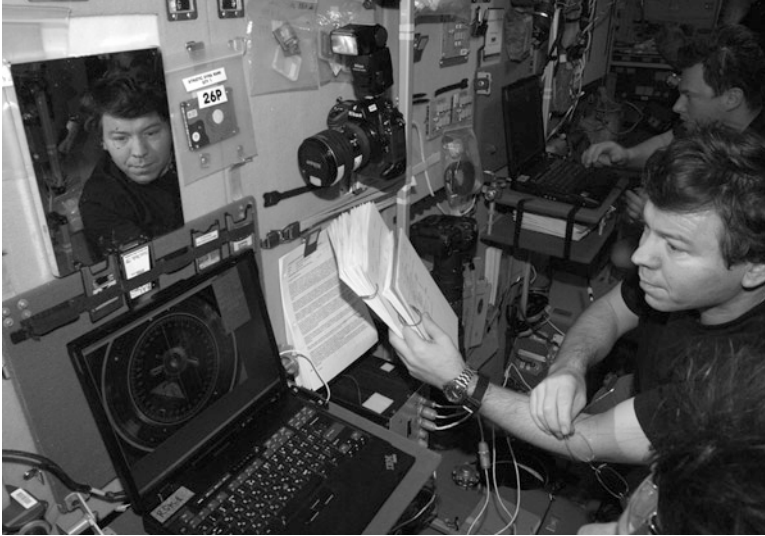
Figure 9.9. Astronauts Use a Laptop-Based Simulator on Board the ISS to Prepare for a Soyuz Relocation Maneuver. Note That They Still Make Heavy Use of Hard Copy Procedure Documents. (Credit NASA).
