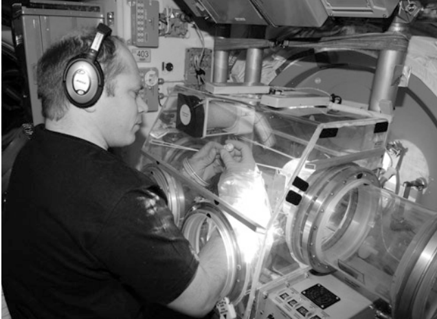
Figure 9.10. An ISS Crewmember Manipulates Hazardous Biological Samples in One of the Gloveboxes of the Russian Research Module. (Credit NASA).
