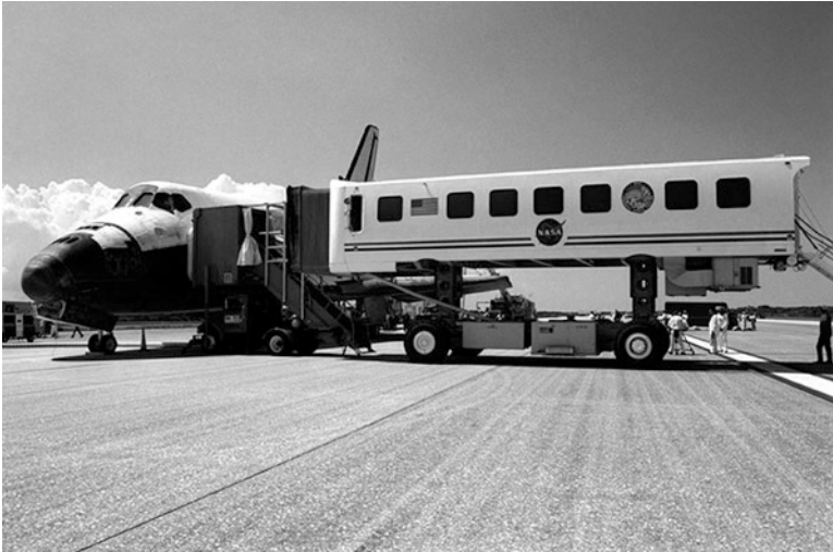
Figure 9.7. The Crew Transport Vehicle Is Docked with the Space Shuttle After Landing. Once Access to the Shuttle Is Possible, Physicians Board the Shuttle and Conduct a Brief Preliminary Examination of the Astronauts. They Assist the Crew in Leaving the Vehicle and Removing Their Launch and Re-entry Suits. (Credit NASA).
