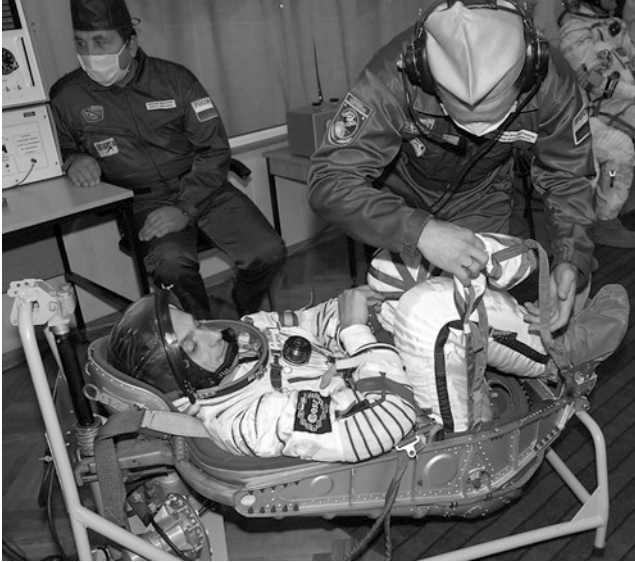
Figure 4.8. During Launch on Board Soyuz, Astronauts Are Reclined on Their Backs in Molded Couches, with Their Legs Higher Than Their Heads. This Prevents Blood from Pooling in the Legs During Ascent and Assists the Heart in Pumping Blood to the Rest of the Body. (Credit NASA).
