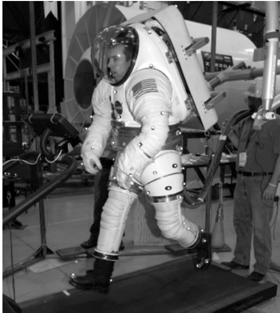
Figure 4.13. Astronaut Performing Treadmill Walking in the Mark-III Prototype EVA Suit. Ground-Based Estimates Suggest That, Depending on the Terrain, Walking on the Lunar and Martian Terrain May Be Difficult and Will Likely Require an Above-Average Aerobic Capacity to Accomplish Safely [Moore et al., 2010]. (Credit NASA).
