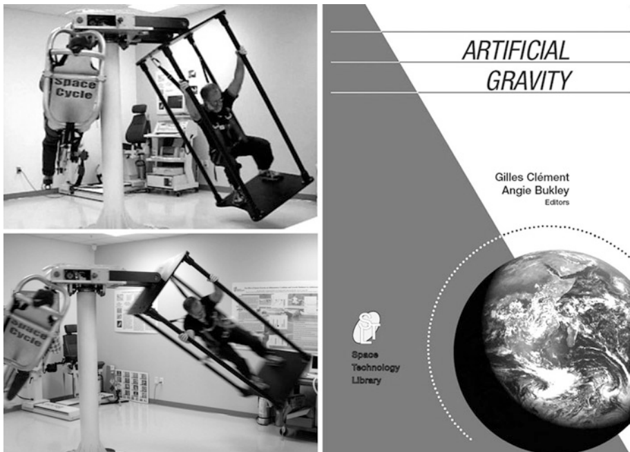
Figure 8.16. To Avoid Some of the Physiological Problems Created By Reduced Gravity, a Continuous or Intermittent Rotating Environment Could Provide an Artificial Gravity Environment, the Level of Which Is Still to be Defined. One Method to Achieve Intermittent Artificial Gravity in the Mars Habitat Is the Space Cycle Proposed by the University of California, Irvine. For More Details, See the Book Artificial Gravity by Clément and Bukley [2007].
