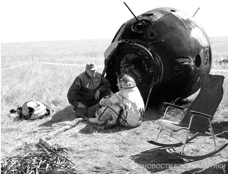
Figure 7.20. One of the Crewmembers of Soyuz TMA-11 Is Chatting with a Member of the Recovery Team After Landing. His Capsule Unexpectedly Followed a High-g Ballistic Re-entry Trajectory and Ended up Landing 400 km Off-Course. (Credit Novosti Kosmonavtiki).
