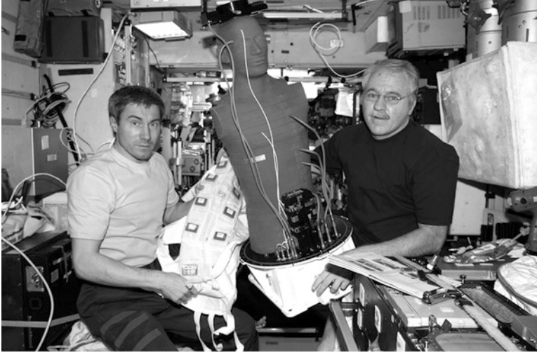
Figure 2.27. ISS Astronauts Display the Phantom Torso That Monitors the Radiation Level at Various Depths Within Its Tissues When Placed Inside or Outside the ISS. (Credit NASA).
