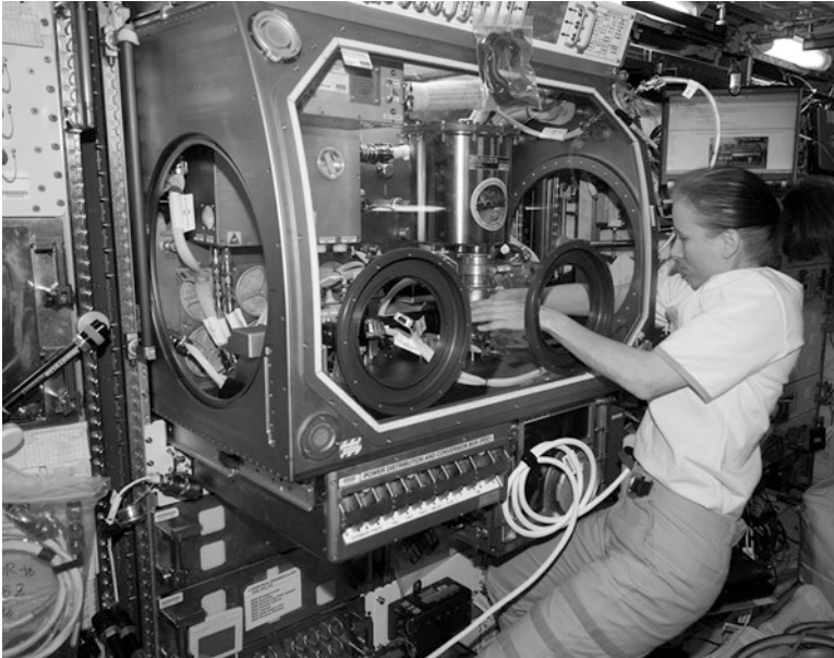
Figure 2.29. An Astronaut Works on a Biology Experiment Inside the Microgravity Science Glovebox (MSG) in the Columbus Laboratory of the ISS. (Credit NASA).
