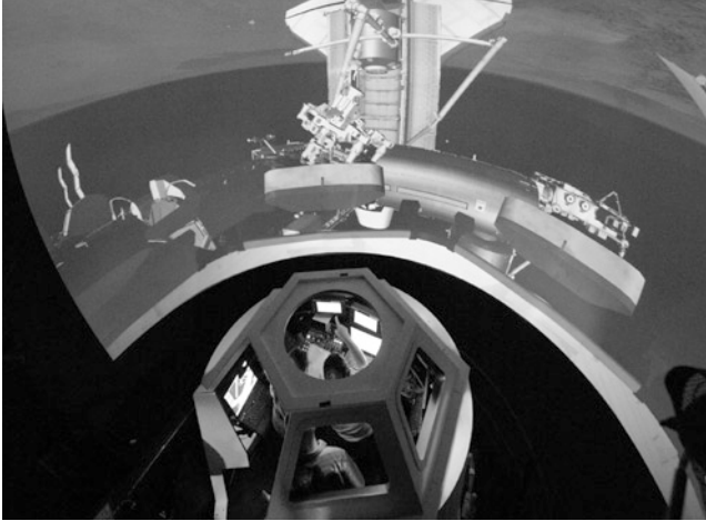
Figure 7.8. Remote Manipulator Arm Training in a Mock-Up of the ISS Cupola and a Surrounding Visual Environment Generated by Virtual Reality. (Credit NASA).
