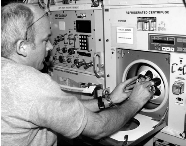
Figure 2.10. A Crewmember Insert Blood Test Samples in a Refrigerated Centrifuge in the Columbus Laboratory of the International Space Station. (Credit NASA).
