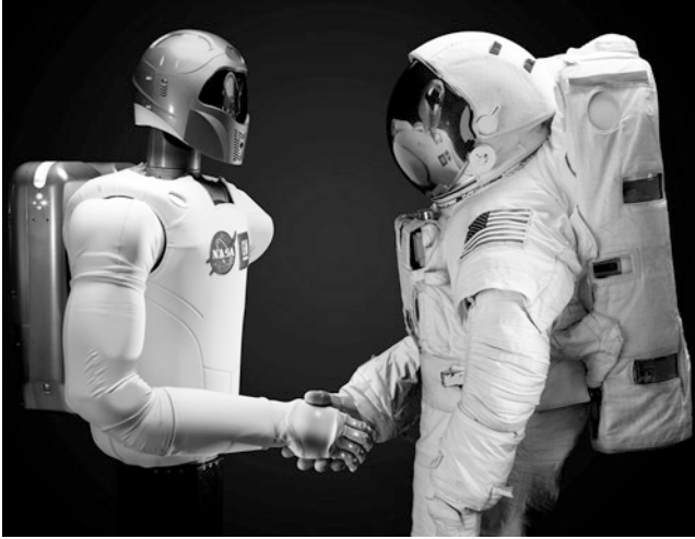
Figure 8.1. Robonaut 2, a Dexterous Humanoid Robot, Will Fly to the ISS on Board STS-133. After Operational Tests and Eventual Upgrades, It Will Help Spacewalking Crew-Members with Tasks Outside the ISS. (Credit NASA).
