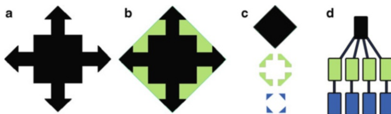
Concavity Tree for Protein–Protein Interaction Analysis, Fig. 1 An object (a), its convex hull with green concavities (b), the actual shape of each node (c) and the corresponding three levels concavity tree (d)
