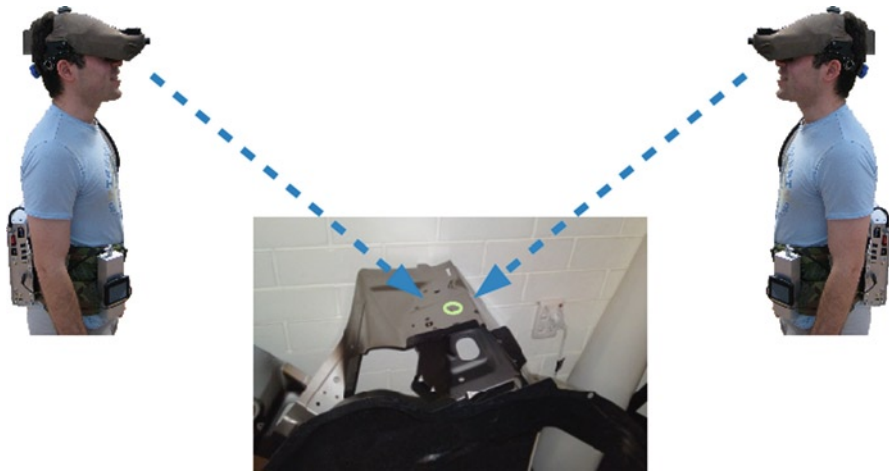
Fig. 4 Concept illustration of combining laser projector-based SAR and HMD-based AR for collaborations
