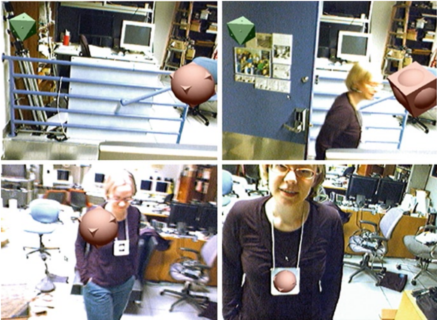
Fig. 1 Frames from a video made using SoundSight. (Top left) Two body-fixed audio elements (green and red), as seen by the local conference participant. (Top right) A remote participant (represented by the red element), using Skype over a Bluetooth headset, enters the room. (Bottom left) The formerly remote participant moves into video tracking range near her audio element. (Bottom right) Her audio element transitions to object-fixed representation (relative to her) when her badge is recognized and tracked
