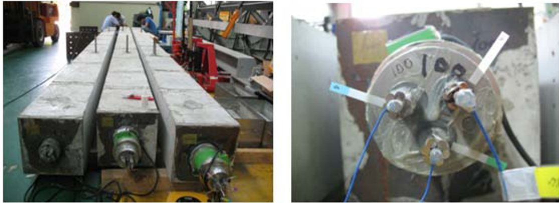
Fig.2 Support Condition and Accelerometer Locations in Test No.4: (a) supports; (b) accelerometers
