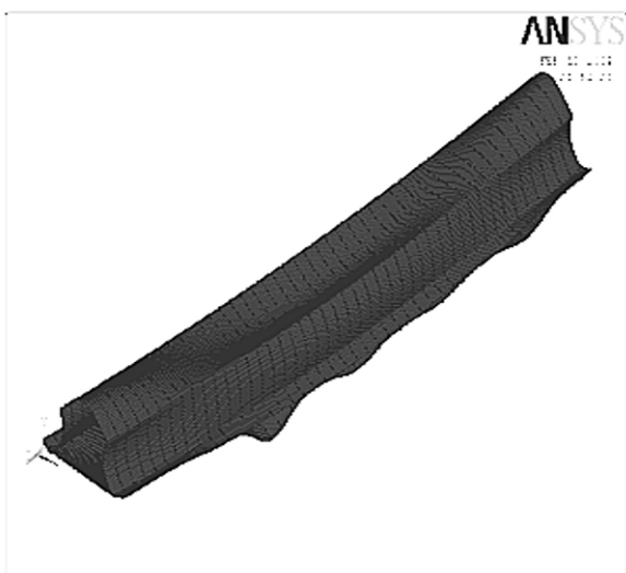
Mode 5 at 873.3 Hz (bending)
