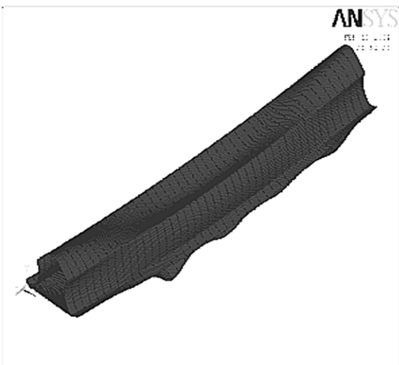
Mode 5 at 873.3 Hz (bending)
