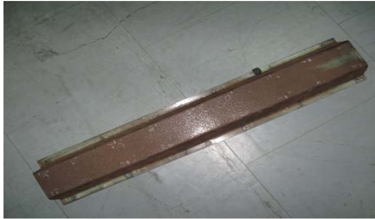
Figure-1 Single hat (SH) structures
