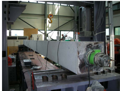
Fig. 1. Post-tensioned concrete beam and load cell
