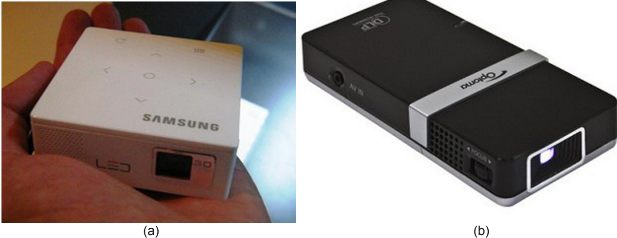
Figure 1. New generation of portable and compact DLP Pico projectors: (a) White Samsung Pico Projector and (b) Optima PK-100.
