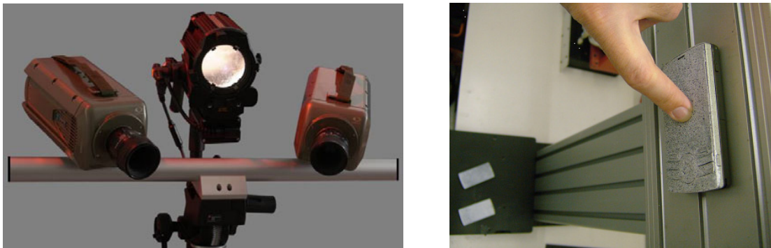
Fig. 5. Setup for the phone drop test (left: high speed cameras; right: test stand).
