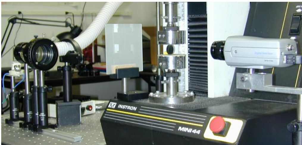
Figure 2. Phase III prototype optical system inspecting silicon disk in compression sample.
