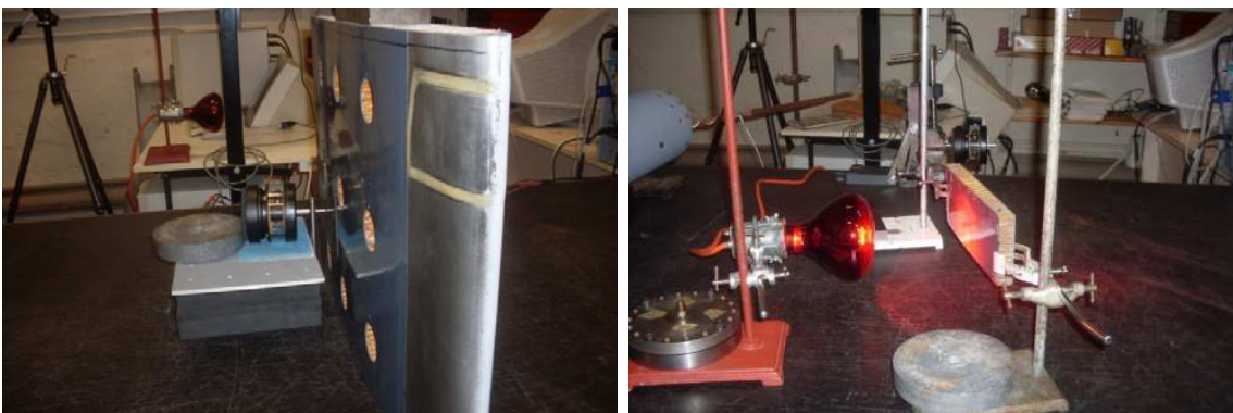
Figure 5. Vibration generator and heating lamp applied to inspection samples.
