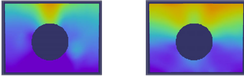
Figure 5a (left): Horizontal Normal Strain for 7075 aluminum insert reinforced joint at 30 kN Figure 5b (right): Vertical Normal Strain for 7075 aluminum insert reinforced joint at 30 kN
