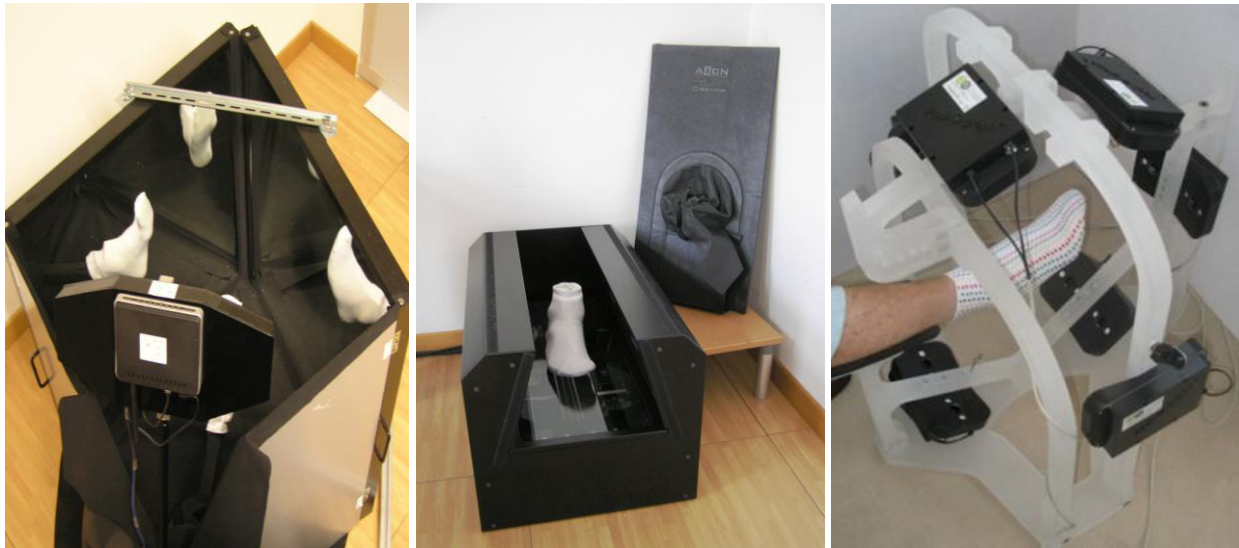
Figure 1. The scanner used for the experiment: silhouette (left), laser (centre) and multiple stereo vision (right) technologies.
