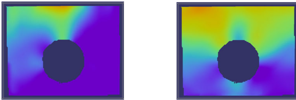
Figure 6a (left): Horizontal Normal Strain for injected insert reinforced joint at 30 kN Figure 6b (right): Vertical Normal Strain for injected insert reinforced joint at 30 kN
