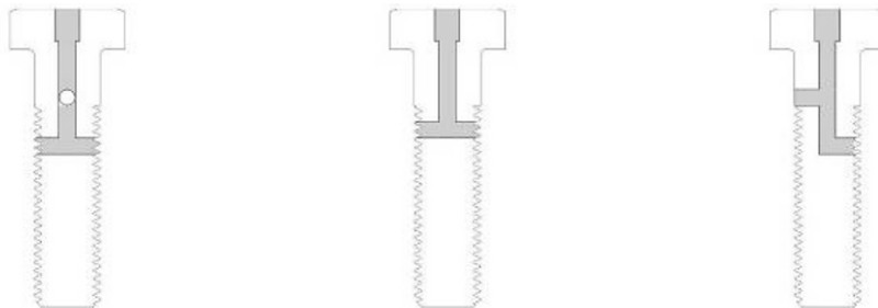
Figure 2: Bolt Configurations (1) Dual Thru-Channel (2) Single Thru Channel (3) Dual Half-Channel
