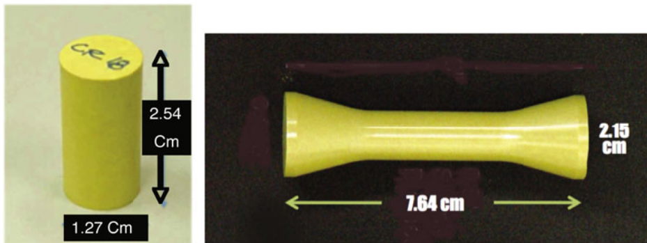
Figure 1 – PBX compression (left) and tension (right) specimens.
