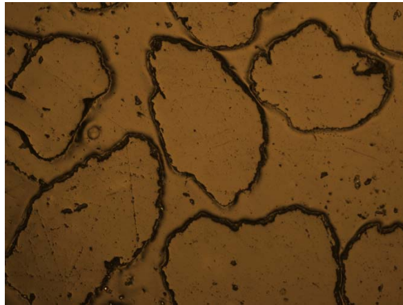
Figure 3. Magnified image of polished sand grains in an epoxy matrix
