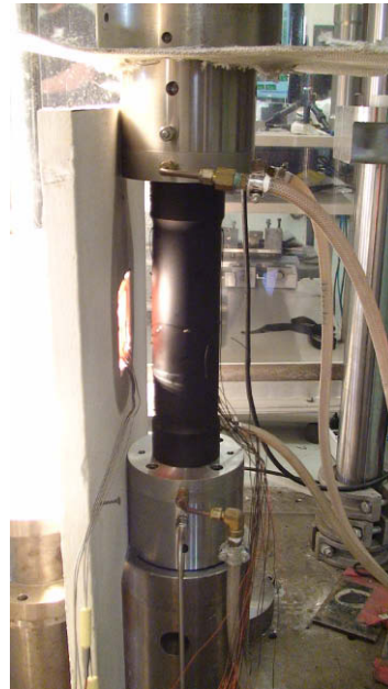
Fig. 4. Photograph of instrumented 304L stainless steel specimen during testing
