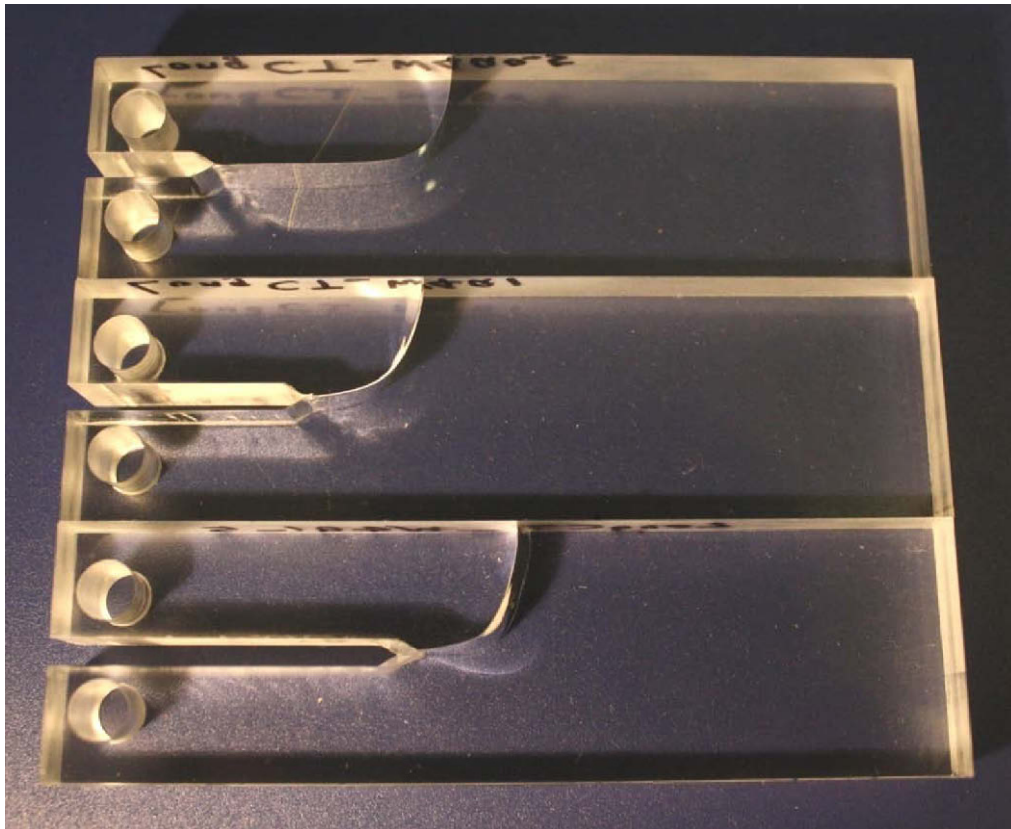
Fig. 6. Trajectories of the crack path of the specimens with different initial crack lengths (From top to bottom: a=12.7 mm, 25.4mm, and 38.1mm.)
