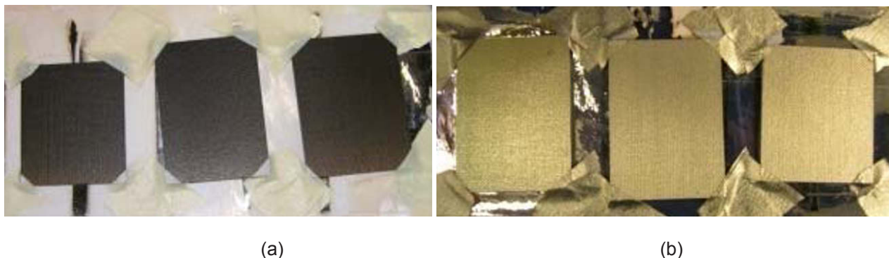
Figure 4: Surface of polyimide composite (a) before and (b) after coating.
