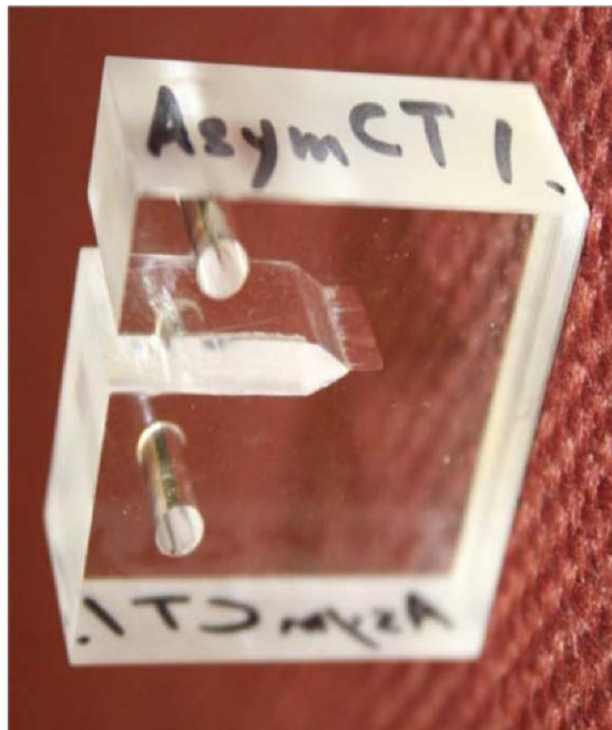
Fig. 5a. Asymmetric CT specimens with notch and initial crack
