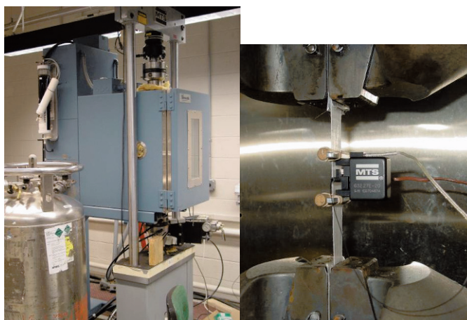
Figure 1: MTS load frame with temperature chamber and lamina sample with extensometer attached.
