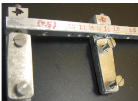
Fig. 1- Custom apparatus used to apply and hold the deformation of aortic specimens.
