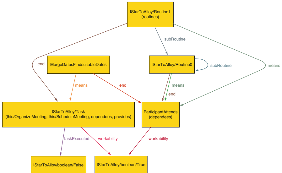
Fig. 5 Example model from running the workability predicate on the case study model
