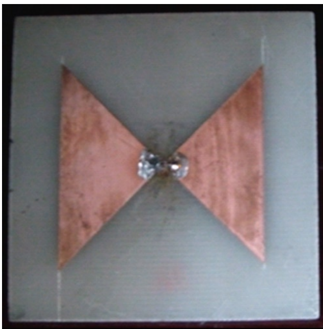
Fig. 5.9 Example of 2D UWB bow-tie antenna
