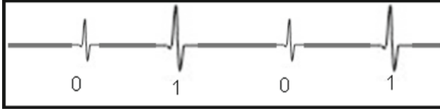
Fig. 3.17 Representation of pulse amplitude modulation (PAM)
