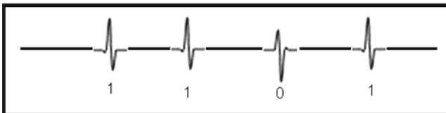
Fig. 3.20 Example of Bi-phase modulation
