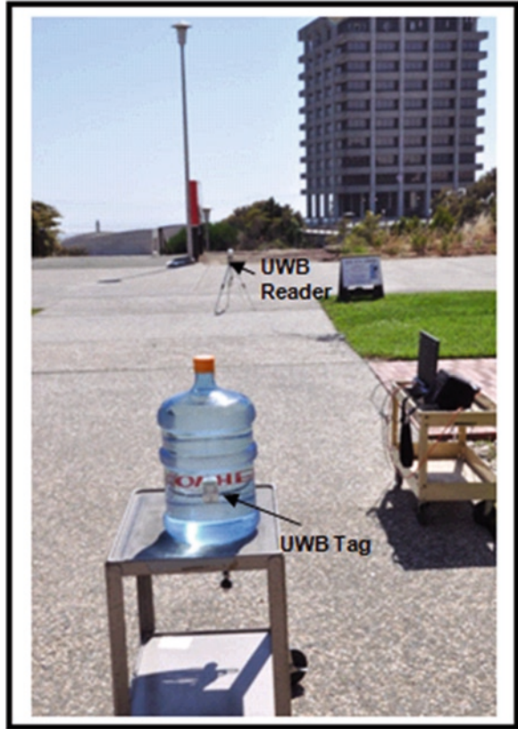
Fig. 3.32 Experimental setup for tag on liquid container
