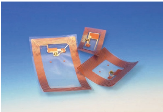
Fig. 1.8 Example of passive tags (courtesy of Texas Instruments, reprinted with permission)
