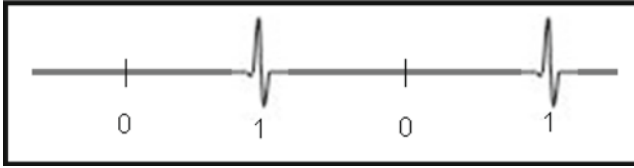
Fig. 3.15 Example of on off keying (OOK) UWB modulation
