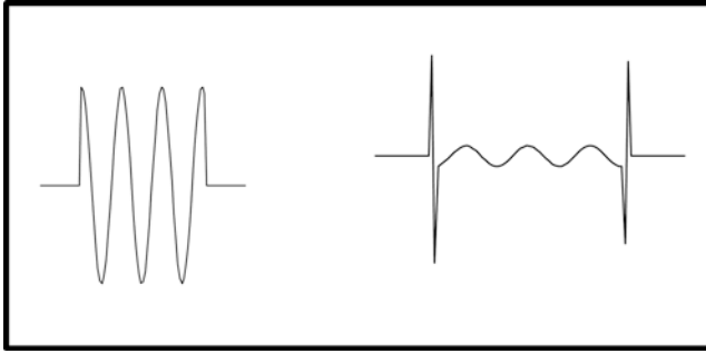
Fig. 4.8 A rectangular box car function ( left ), its and its second derivative ( right )
