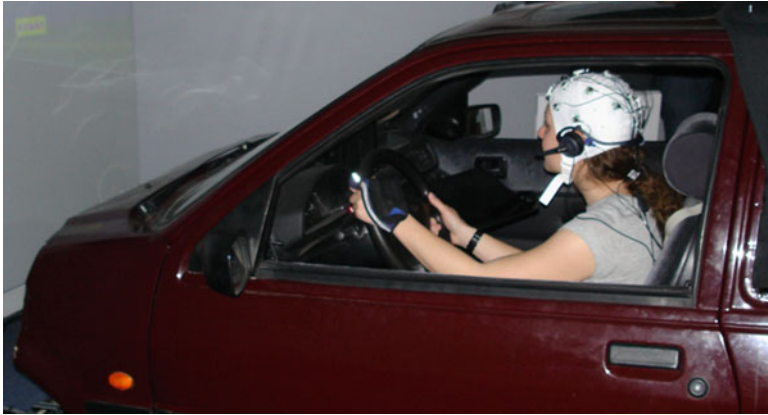
Fig. 8.2 (Part of) the recording setup with EEG cap, audio headset, and sensor glove in the driving simulator
