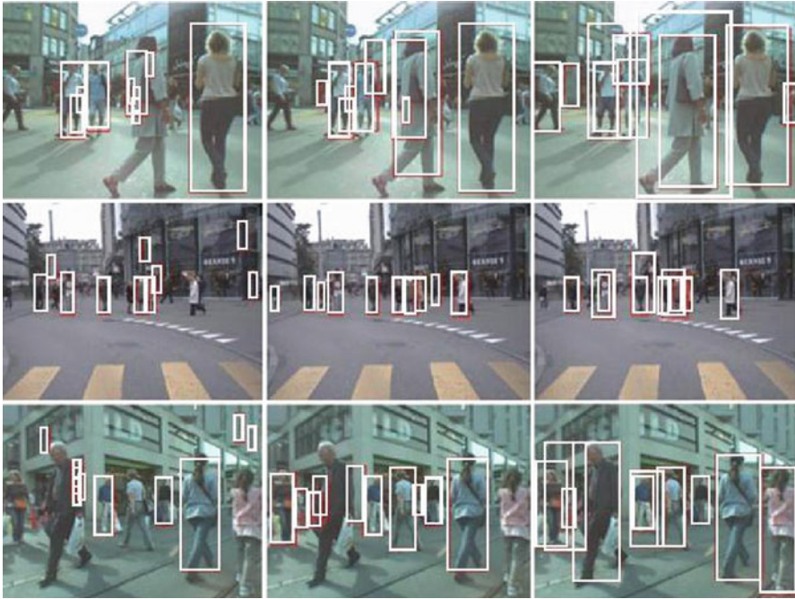
Fig. 16.4 Experimental results: ( left ) baseline system, ( middle ) integration system, ( right ) UoCTTI system
