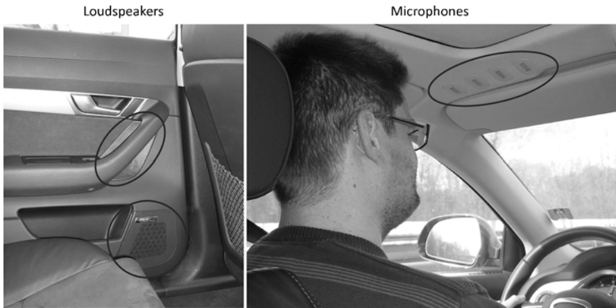
Fig. 5.3 Positioning of loudspeakers and microphones (With permission from SVOX)
