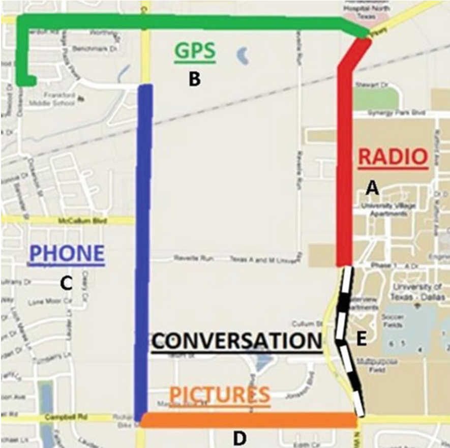
Fig. 18.3 Route used for the recording (5.6 miles long). Subjects drove this route two times. In the first lap, the subjects performed the tasks in order, starting with the Radio task and ending with the Conversation task. In the second lap, the subjects drove the same route without performing any task. The second lap involves normal driving without any of the aforementioned tasks, which is used as a normal reference. Since the same route is used for both normal and task conditions, the analysis is less dependent on the selected road
