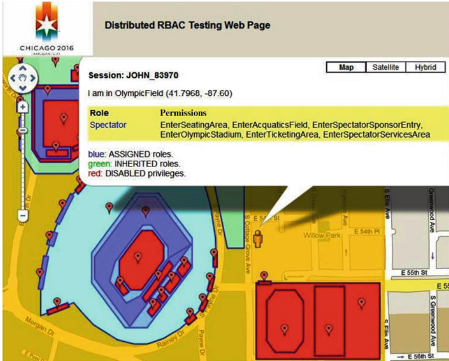
Fig. 6.8 Visual interface showing areas, users, permissions, and roles. Unaccessible areas are shown in red
