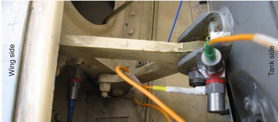
Figure 6: Instrumentation of the rear attachment of the right wing.
