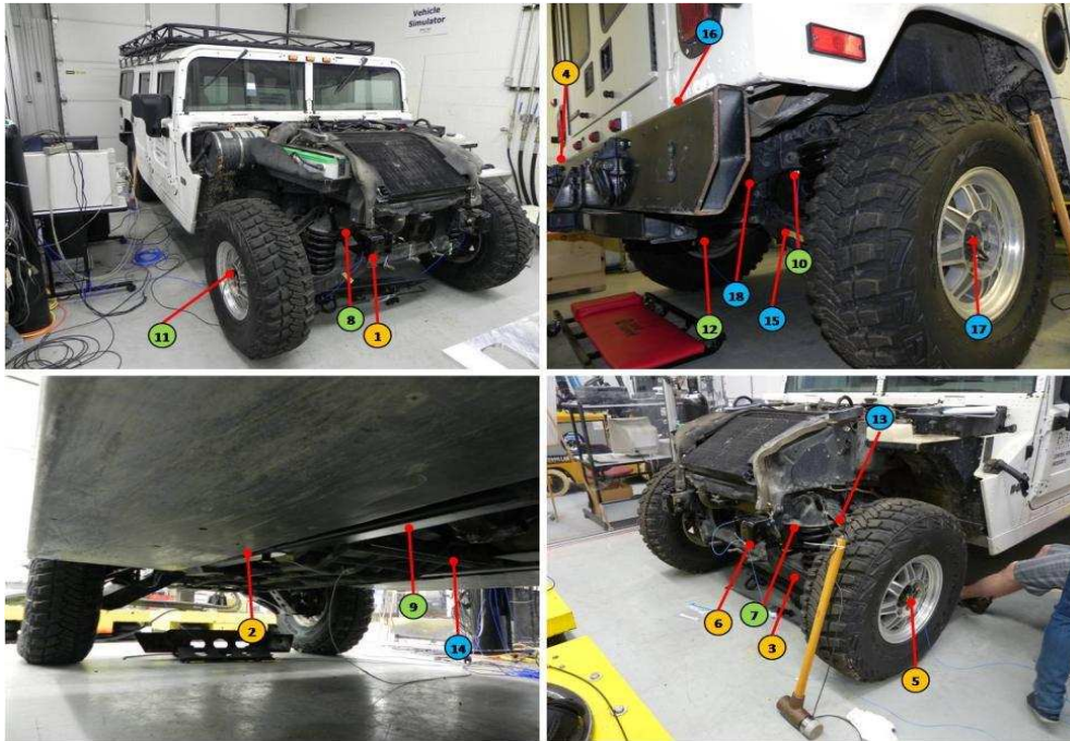
Fig. 3 Sensor locations for each measurement set
