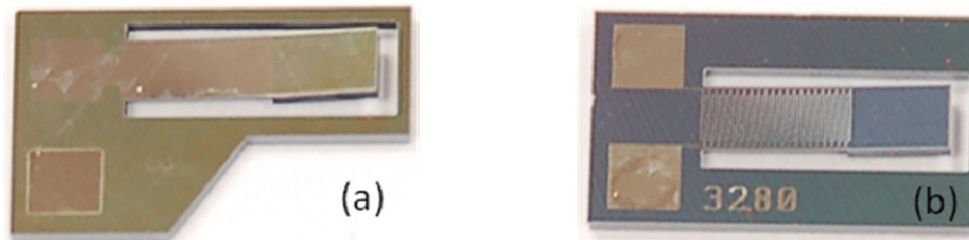
Figure 4: Photographs of the fabricated energy harvesting devices that have (a) 31 mode and (b) 33 mode.
