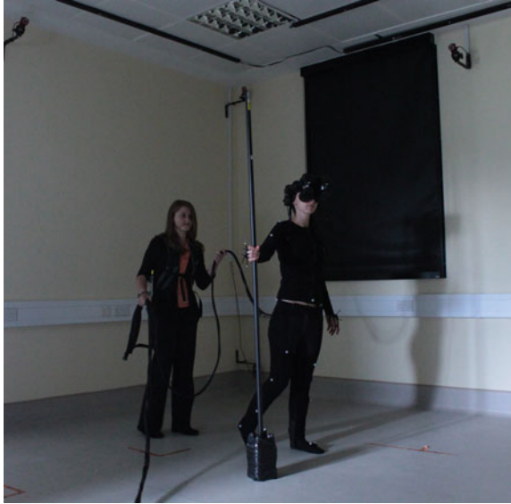
Fig. 7.12 A user wearing a motion capture suit within an OptiTrak installation. The user is taking part an experiment involving a simulation of a train. Courtesy of Angus Antley, University College London
