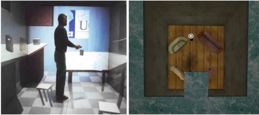
Fig. 7.3 Left UCL's four-walled CAVE™-like display. Right looking down into the virtual pit
