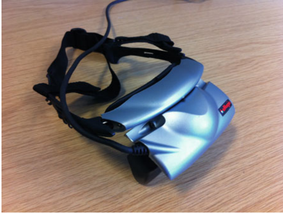
Fig. 7.11 The eMagin z800 helmet contains a three axis rotation sensor
