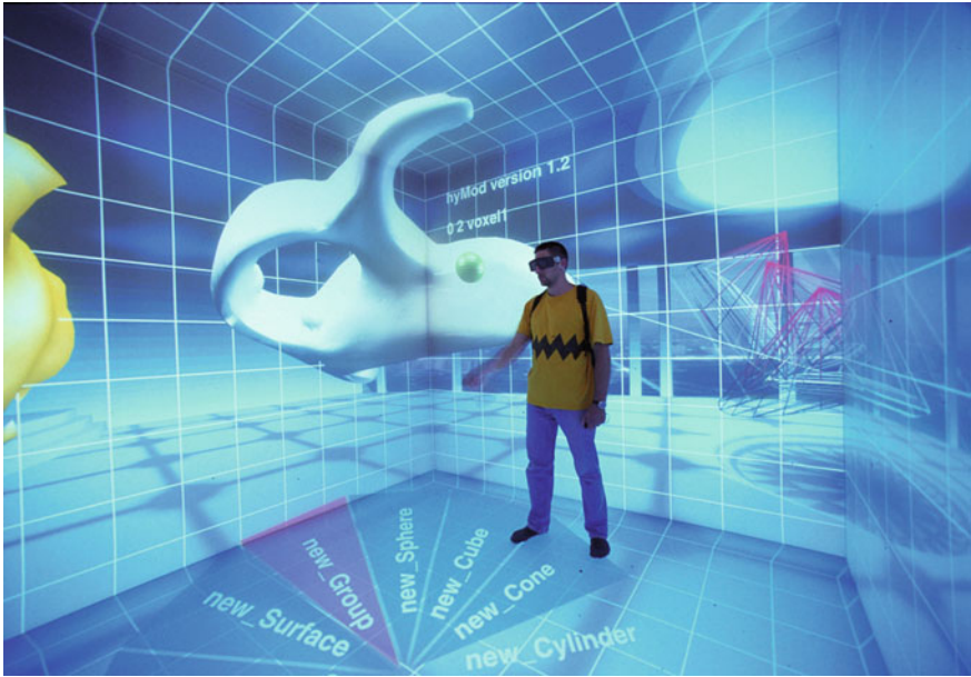
Fig. 7.4 HyPi-6 display at the Fraunhofer IAO, Stuttgart, Germany. Courtesy of Oliver Stefani
