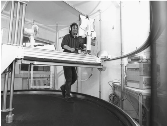
Fig. 6.2 The circular treadmill (CTM) at the Max Planck Institute for Biological Cybernetics. It consists of a large motorized wooden disc ( \varnothing = 3.6\text{ m} ) covered with a slip resistant rubber surface and a motorized handlebar. The disc and handlebar can be actuated independently from each other. The disc's maximum angular velocity is 73^\circ/\text{s} , and the handlebar can reach a maximum velocity of 150^\circ/\text{s} . Walking on the CTM is natural and intuitive and does not require any explicit training (see also [42]). For the overground versus treadmill study (Sect. 6.2.2) the setup was equipped with a TrackIR: Pro 4 (NaturalPoint) optical tracking device for tracking the position and orientation of the head. It was fixed on top of the depicted laptop monitor that was mounted in front of the participant. The device has a 46^\circ field of view and provides 6 DOF tracking with mm and sub-degree precision for position and orientations, respectively. For the experiments described in Sects. 6.3.2 and 6.2.3, a custom-built pointing device was mounted on the handlebar within comfortable reaching distance of the right hand (at a radius of 0.93\text{ m} from the center of the disk). The pointing device consisted of a USB mechanical rotary encoder (Phidgets, Inc.) with a pointing rod attached and encased in plastic (see also [42]). Note that the CTM has since moved to the department of Cognitive Neurosciences at Bielefeld University. (Photograph courtesy of Axel Griesch)
