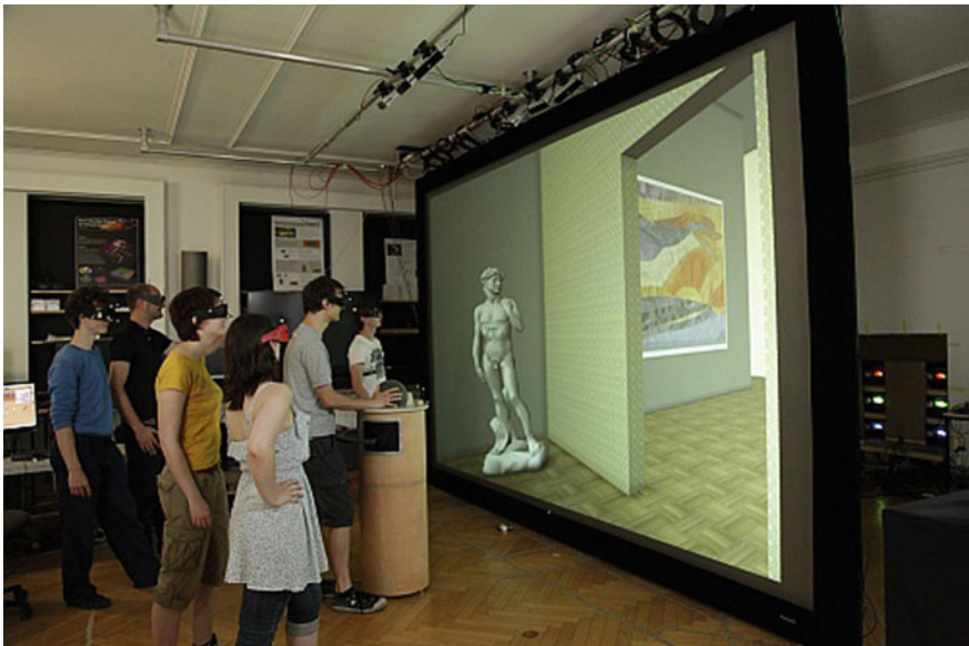
Fig. 7.2 The C1X6 supports six users, each seeing a first person stereo view [15]. Courtesy of Virtual Reality Systems Group, Bauhaus-Universität Weimar, Germany
