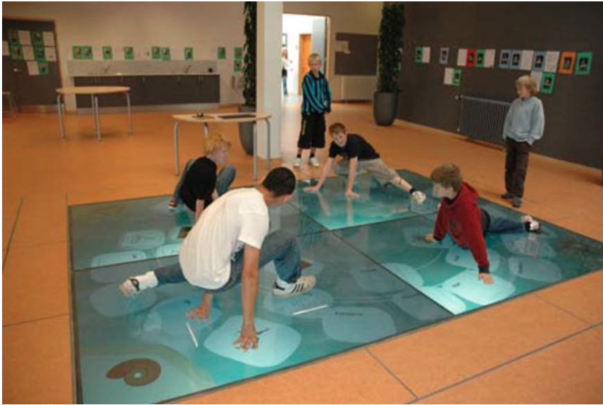
Fig. 17.5 The iGameFloor interface of Gronboek et al. [12] uses vision-based limb tracking on a rear-projected interactive floor comprised of back-projected translucent floor plates (image reproduced from [12])
