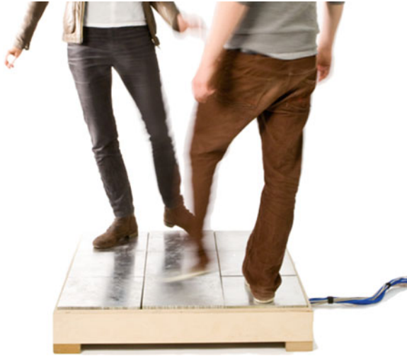
Fig. 17.8 Example of a portable, 9-tile version of the distributed floor interface of Visell et al. [39], shown without video feedback, as developed by Kemper, Franinovic, Wille, and Visell
