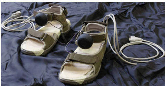
Fig. 12.9 Photo of the actuated shoes [77] with loudspeakers mounted on the top . The cable in the foreground interfaces the sensors in the shoes with the data acquisition unit
