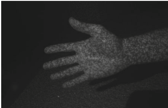
Fig. 16.6 The structured light pattern generated by the Kinect's infrared laser projector is shown. Through stereo triangulation between two images, a depth map is constructed
