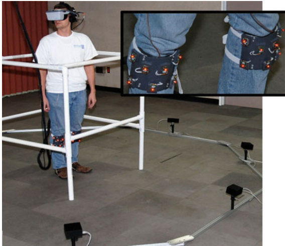
Fig. 11.5 GUD-WIP in use. The user is free to maneuver and rotate within the PVC pipe “cage” that constrains his motion and protects the cameras. The beacons on the user’s shins (inset) are sensed by the eight PhaseSpace cameras arrayed around the user. Data from knee tracking is used for both speed and the direction setting. The HMD and head-tracker have wired connections; the PhaseSpace system is wireless. (Reproduced from Wendt [40])
