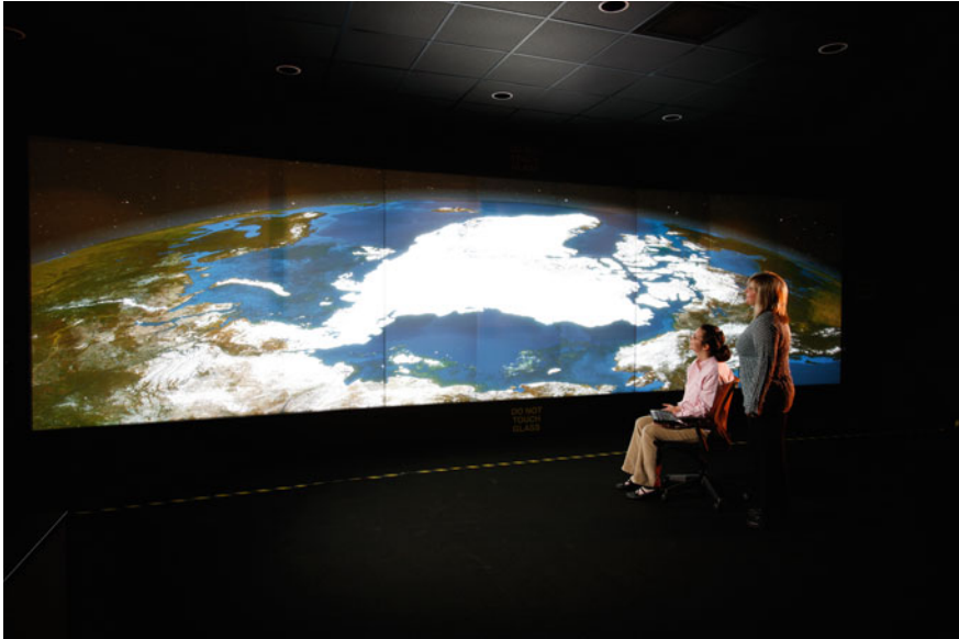
Fig. 7.1 An example of a wall-sized display. The EVEREST display is 30 ft long by 8 ft tall and displays 35 million pixels. Image courtesy of the National Center for Computational Sciences, Oak Ridge National Laboratory
