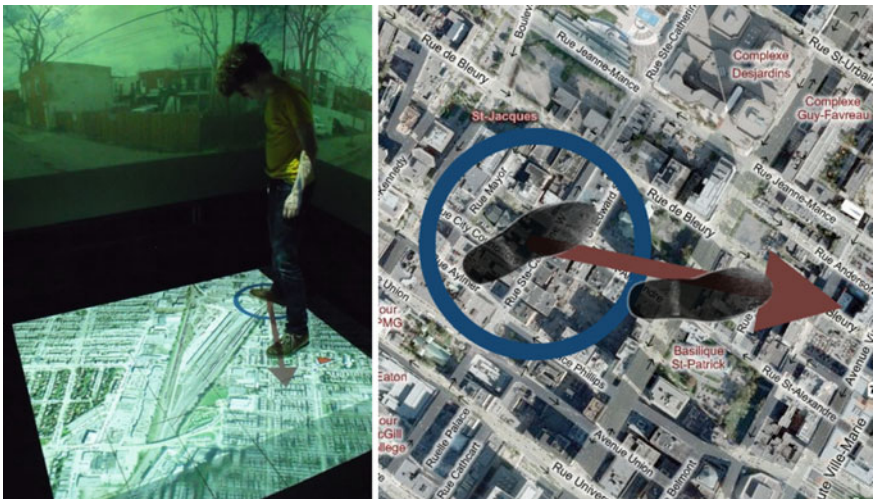
Fig. 17.15 The first foot to remain still establishes the pivot point, surrounded by a blue circle. The second foot then specifies the vector, relative to the pivot, for panning
