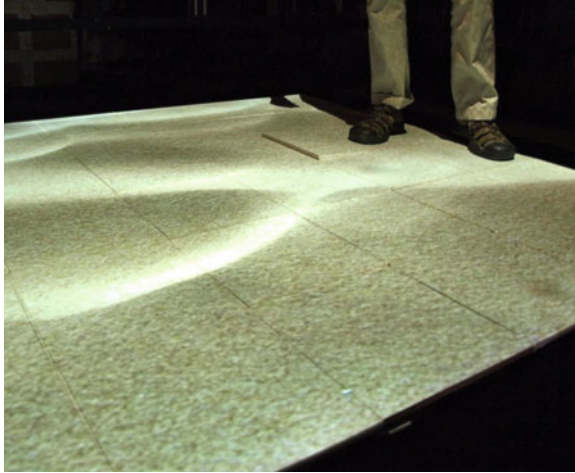
Fig. 17.1 A floor interface situated within an immersive, rear projected virtual environment simulator
