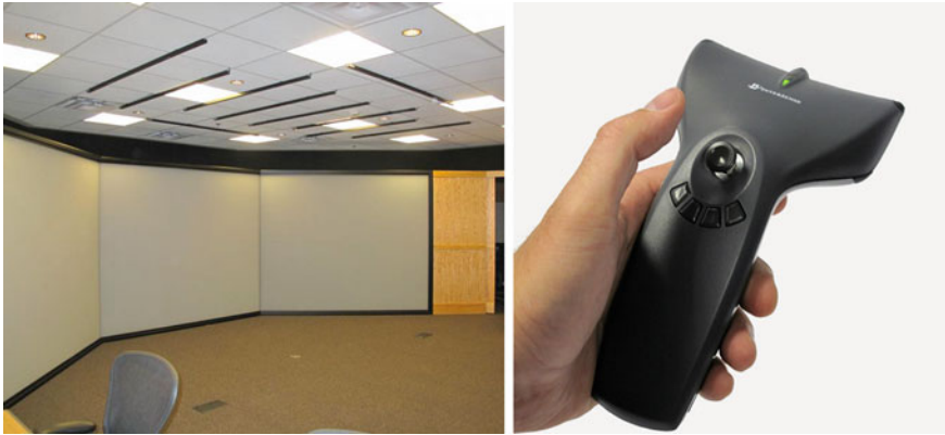
Fig. 7.13 Left a typical Intersense IS900 sensor bar installation. Right Intersense IS9000 MicroTrax Wand. Courtesy of Intersense, LLC
