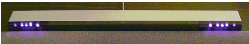
Fig. 16.2 The Wiimote sensor bar has two groups of IR LEDs at fixed widths
