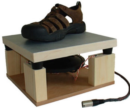
Fig. 12.8 Photo of an actuated tile with large mens' shoe, showing representative size. The model shown is based on the low-cost force sensing resistor option. The cable in the foreground interfaces the sensors with the data acquisition unit
