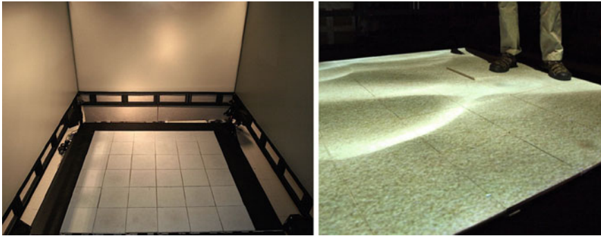
Fig. 17.6 The floor interface is situated within an immersive, rear-projected virtual environment simulator. Right visual feedback is provided by top-down video projection (in the instance shown, this corresponds to a virtual, multimodal sand scenario—see Chap. 12)
