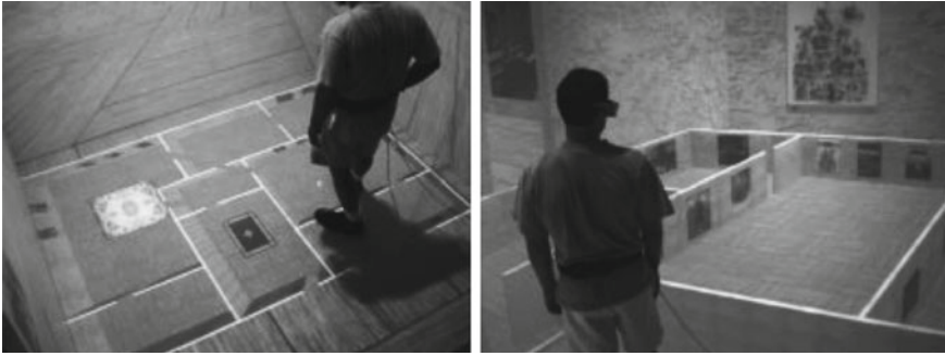
Fig. 17.3 The step WIM interface of LaViola et al. introduced an interactive floor display for navigating within a virtual environment via foot gestures performed with instrumented shoes [19]
