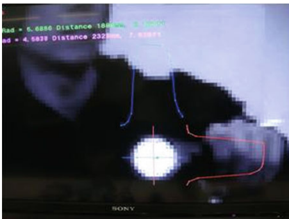
Fig. 16.4 Visualizing the 2D pixel intensity distribution of the Move's sphere is useful for debugging the model fitting stage
